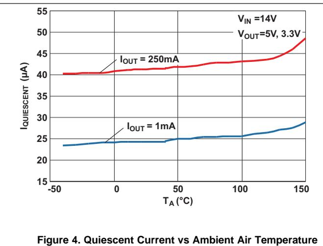
Figure 4. Quiescent Current vs Ambient Air Temperature
