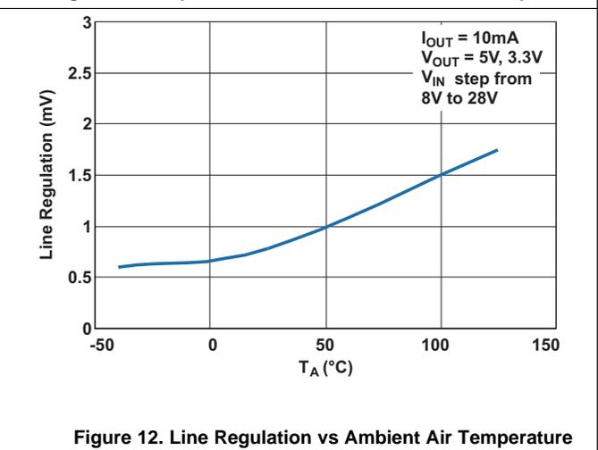
Figure 12. Line Regulation vs Ambient Air Temperature
