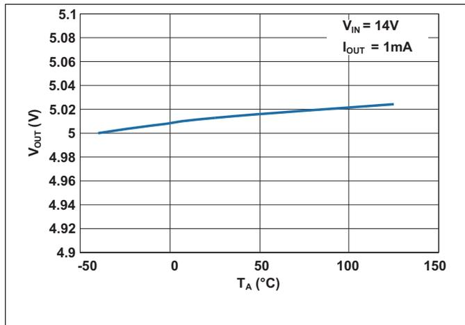
Figure 7. Output Voltage vs Ambient Air Temperature
