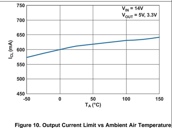
Figure 10. Output Current Limit vs Ambient Air Temperature
