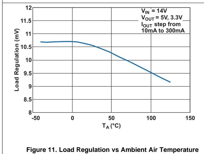
Figure 11. Load Regulation vs Ambient Air Temperature
