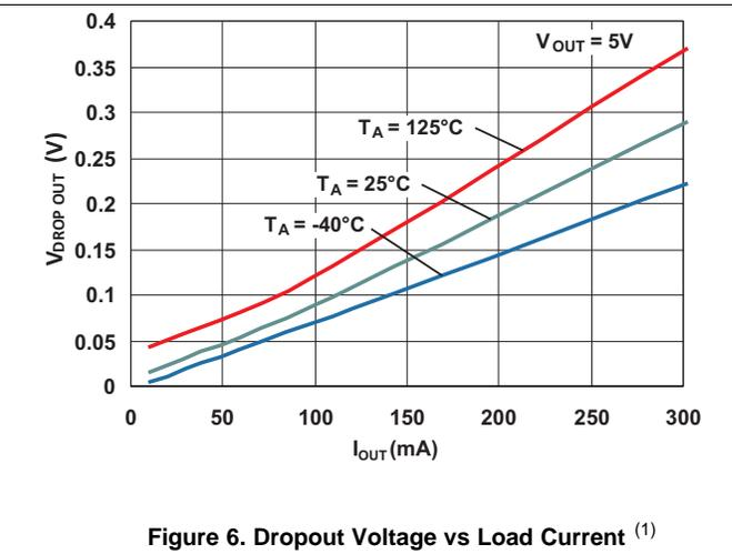
Figure 6. Dropout Voltage vs Load Current <sup>(1)</sup>
