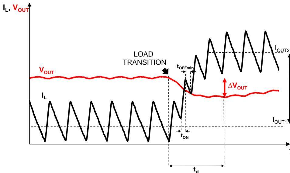
The selection of the  $C_{OUT}$  is related to the  $t_d$  as well as to the current step  $\Delta I_{OUT}$  and the max allowed voltage drop  $\Delta V_{OUT}$ , as shown by the following equation:
