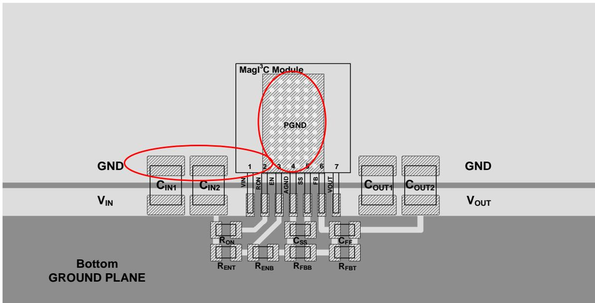
The negative terminal of  $C_{IN1}$  and  $C_{IN2}$  needs to be very close to the PGND pad of the power module.
