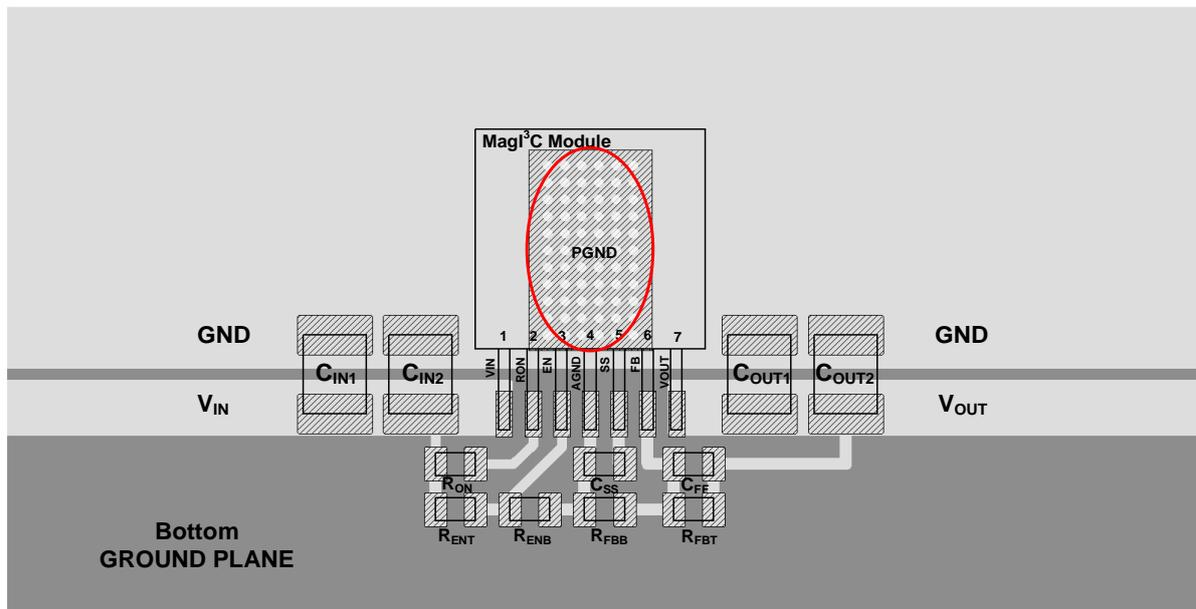
Place a dedicated PGND copper area beneath the MagI<sup>3</sup>C Power Module. Use an array of heat-sinking vias to connect the PGND pad to the ground plane on the bottom PCB layer. If the PCB has multiple of copper layers, these thermal vias can also be used to make a connection to the heat-spreading ground planes located on inner layers.
