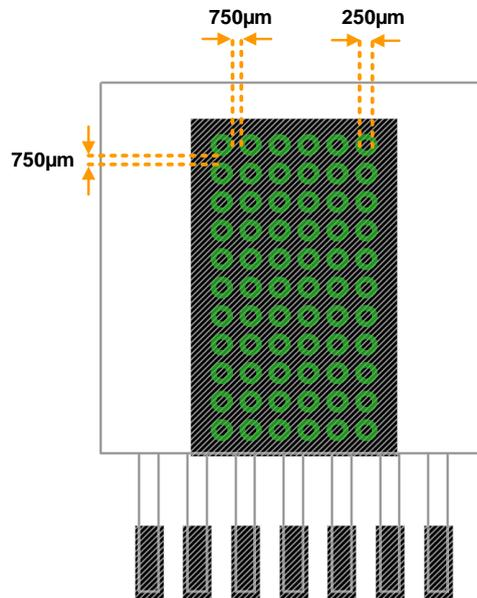
For best result, use a thermal via array as proposed in the picture above with drill of max 250µm, spaced 750µm apart. Ensure enough copper area is used for heat-sinking, to keep the junction temperature below 125°C.
