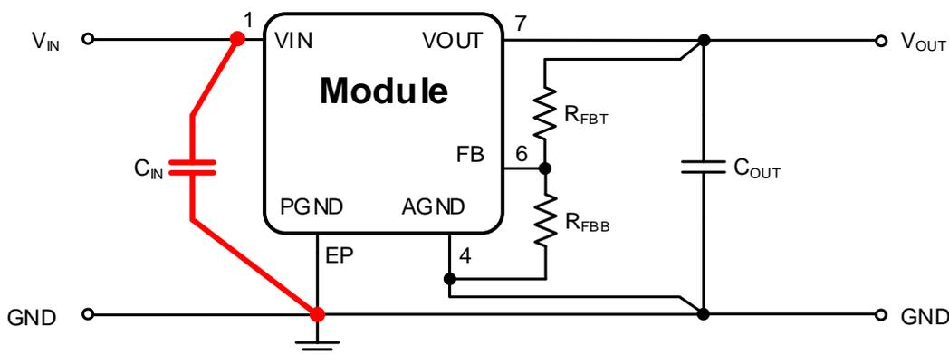
Based on those considerations, the path of the input capacitor  $C_{IN}$  is the most critical one to generate high frequency noise on  $V_{IN}$ . Therefore place  $C_{IN}$  as close as possible to the MagI<sup>3</sup>C power module  $V_{IN}$  and PGND exposed pad EP. This will minimize the high di/dt area and reduce radiated EMI. Additionally, grounding for both the input and output capacitor should consist of a localized top side plane that connects to the PGND exposed pad.
