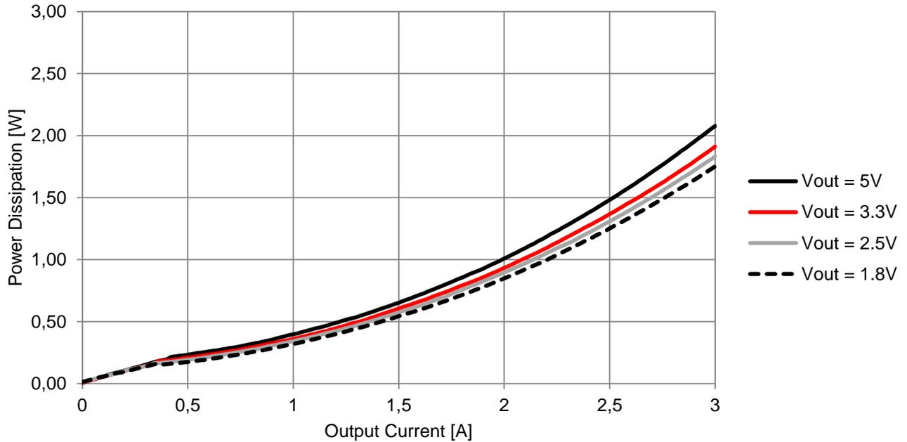
171030601  $V_{IN} = 12V$ ,  $f_{SW} = 500kHz$ ,  $T_A = 85^\circ C$
