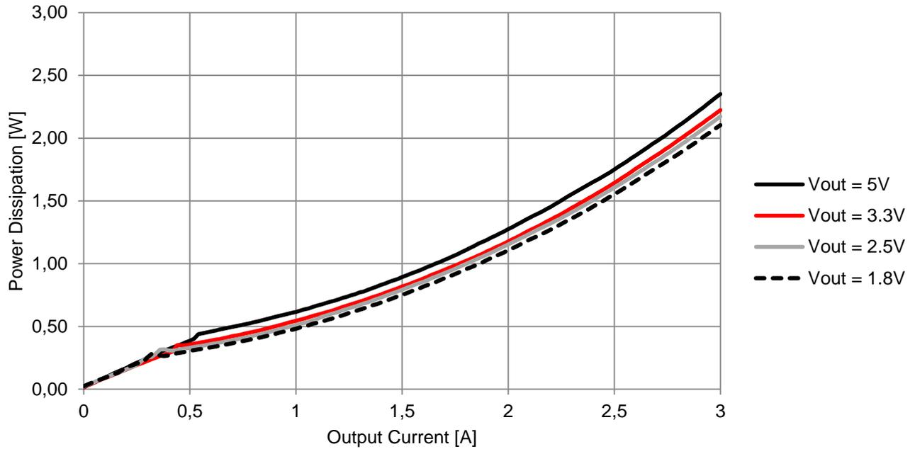
171030601  $V_{IN} = 24V, f_{SW} = 500kHz, T_A = 85^\circ C$
