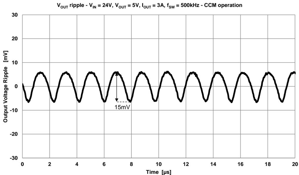
The output voltage ripple during CCM operation is much lower ( $<15mV_{pp}$ ) than the ripple during DCM operation (around  $35mV_{pp}$ ).
