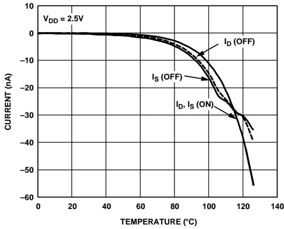
Figure 10. Leakage Currents vs. Temperature,  $V_{DD} = 2.5\text{ V}$
