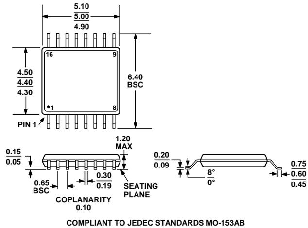
Figure 27. 16-Lead Thin Shrink Small Outline Package [TSSOP] (RU-16)
