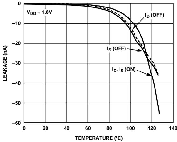
Figure 11. Leakage Currents vs. Temperature,  $V_{DD} = 1.8\text{ V}$
