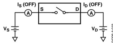
Figure 19. Off Leakage
