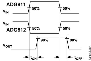
Figure 21. Switching Times
