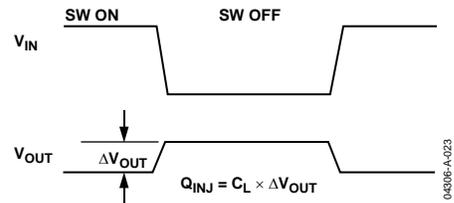
Figure 23. Charge Injection
