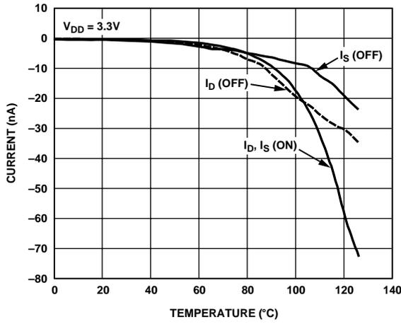
Figure 9. Leakage Currents vs. Temperature,  $V_{DD} = 3.3\text{ V}$
