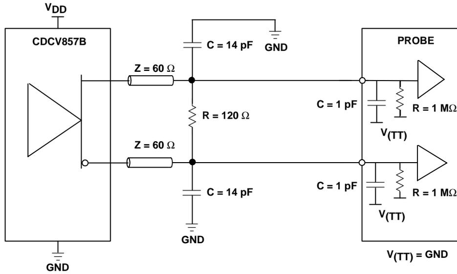
Figure 3. Output Load Test Circuit for Crossing Point
