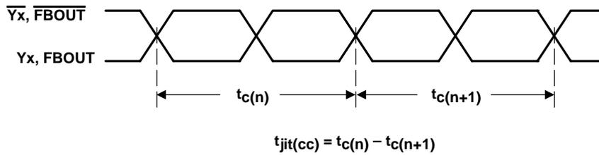
Figure 4. Cycle-to-Cycle Jitter
