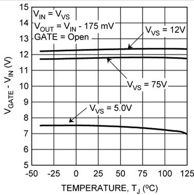
Figure 13.  $V_{GATE} - V_{IN}$  vs Temperature
