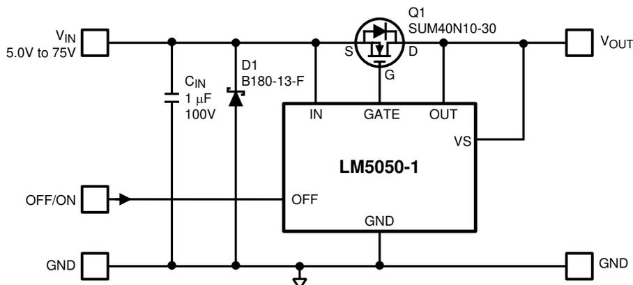
Figure 30. Basic Application With Input Transient Protection Schematic
