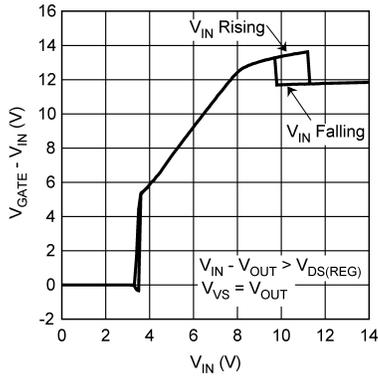
Figure 9. ( $V_{GATE} - V_{IN}$ ) vs  $V_{IN}$ ,  $V_{VS} = V_{OUT}$
