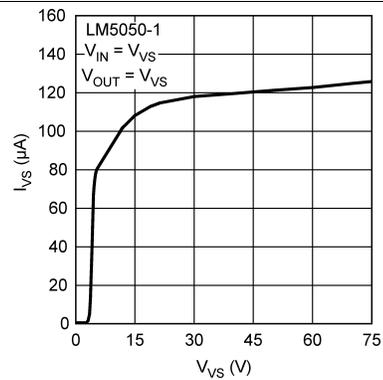
Figure 8.  $I_{VS}$  vs  $V_{VS}$
