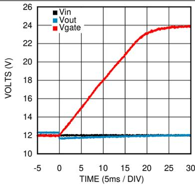
Figure 11. Forward  $C_{GATE}$  Charge Time,  $C_{GATE} = 47\text{ nF}$
