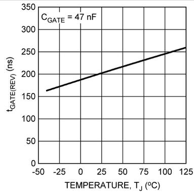
Figure 14.  $t_{GATE(REV)}$  vs Temperature
