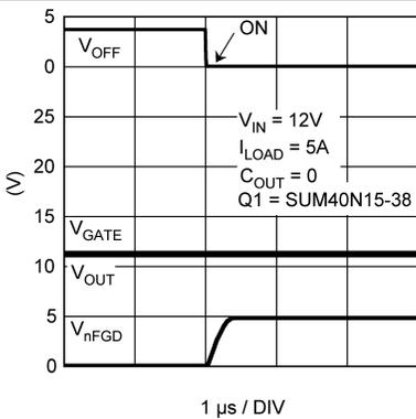
Figure 19. OFF Pin, OFF to ON Transition
