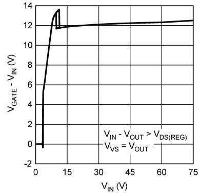
Figure 10. ( $V_{GATE} - V_{IN}$ ) vs  $V_{IN}$ ,  $V_{VS} = V_{OUT}$
