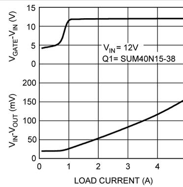
Figure 20. GATE Pin vs  $(R_{DS(ON)} \times I_{DS})$
