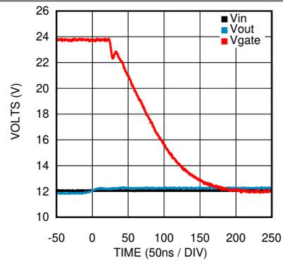
Figure 12. Reverse  $C_{GATE}$  Discharge,  $C_{GATE} = 47\text{ nF}$
