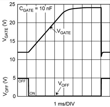
Figure 17.  $C_{GATE}$  Charge and Discharge vs OFF Pin
