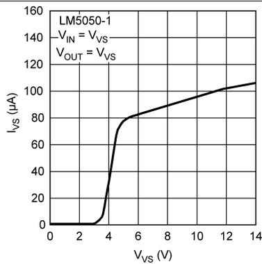
Figure 7.  $I_{VS}$  vs  $V_{VS}$
