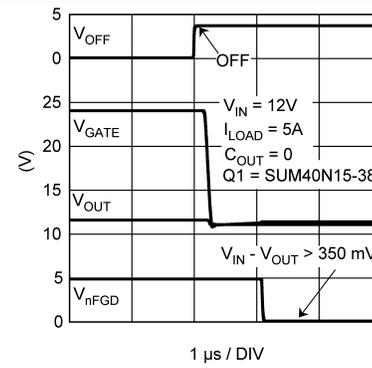
Figure 18. OFF Pin, ON to OFF Transition
