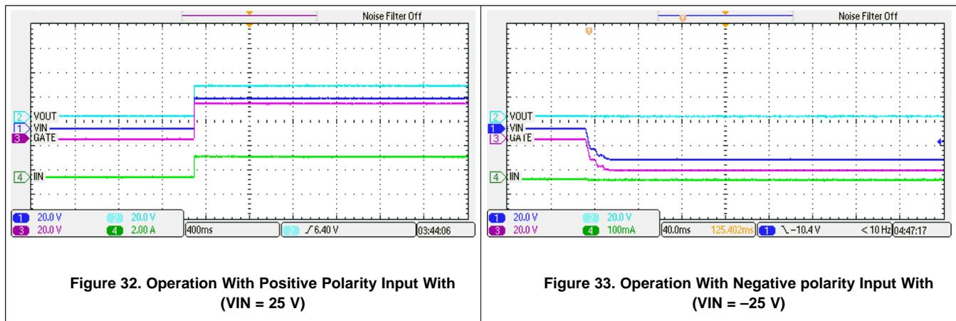
Figure 32. Operation With Positive Polarity Input With ( $V_{IN} = 25\text{ V}$ )
