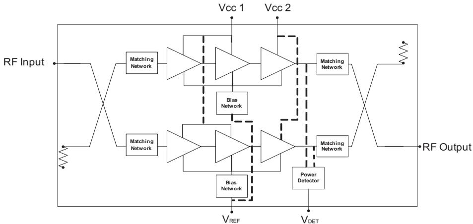
**Figure 1: Block Diagram**
