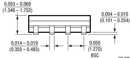
\*DIMENSION DOES NOT INCLUDE MOLD FLASH. MOLD FLASH SHALL NOT EXCEED 0.006" (0.152mm) PER SIDE
