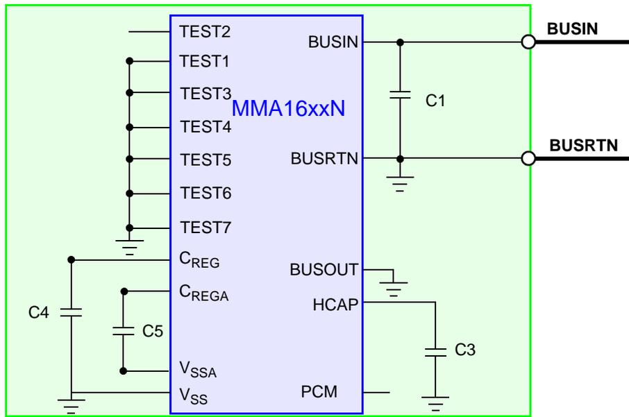
Figure 1. Application Diagram
