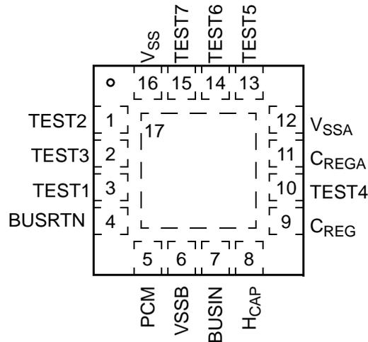
Figure 4. Pinout
