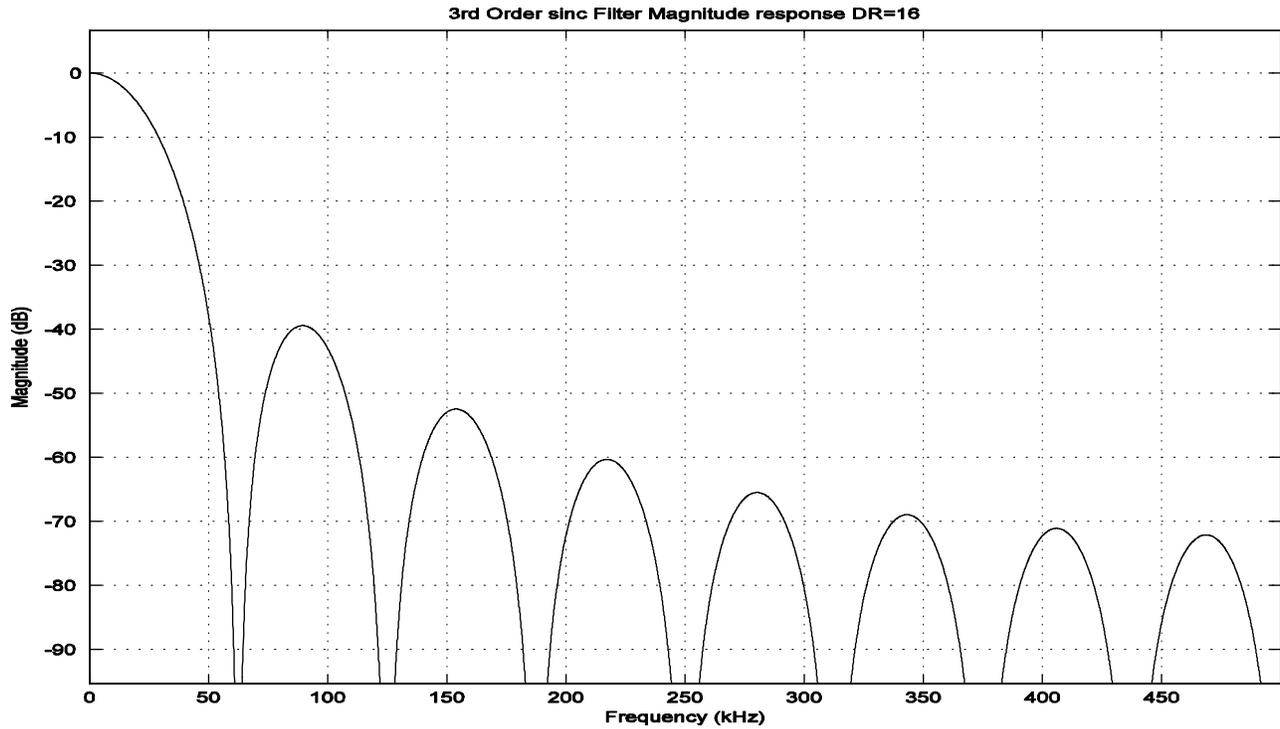
Figure 14. Sinc Filter Response,  $t_s = 16 \mu s$
