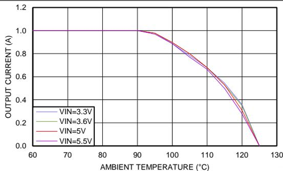
**Figure 3. Thermal Derating  $V_{OUT} = 1.8\text{ V}$ ,  $\Theta_{JA} = 77^\circ\text{C/W}$**
