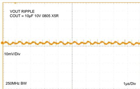
Figure 27. Output Ripple  $V_{OUT} = 2.5 V$
