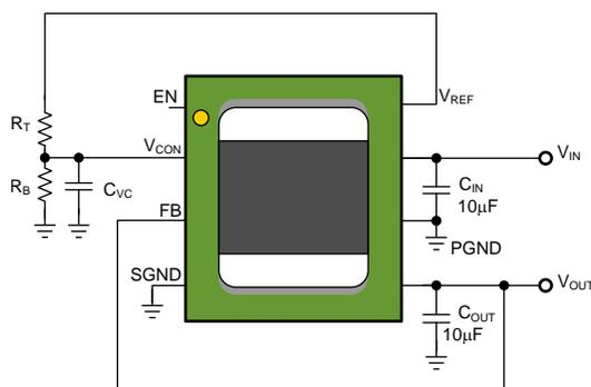
**Figure 12. Typical Application Circuit**
