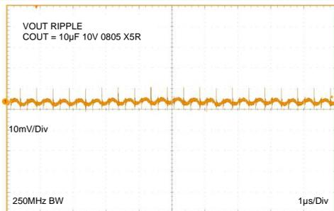
Figure 21. Output Ripple  $V_{OUT} = 1.8\text{ V}$
