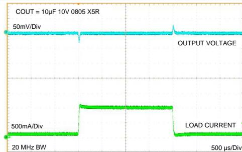
Figure 22. Load Transient  $V_{OUT} = 1.8\text{ V}$
