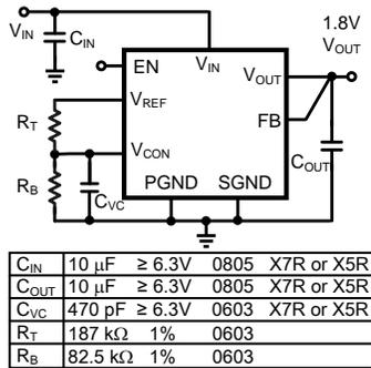
Figure 19. Schematic  $V_{OUT} = 1.8\text{ V}$
