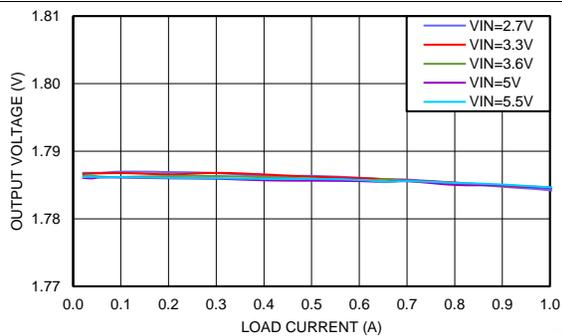
Figure 23. Line and Load Regulation  $V_{OUT} = 1.8\text{ V}$
