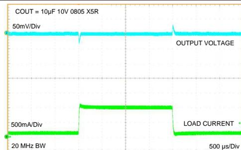
Figure 34. Load Transient  $V_{OUT} = 3.3\text{ V}$
