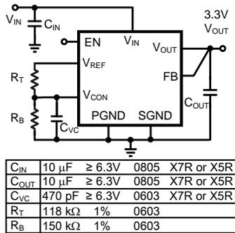
Figure 31. Schematic  $V_{OUT} = 3.3\text{ V}$
