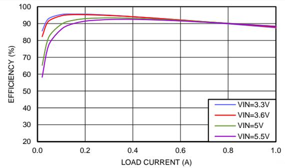
Figure 26. Efficiency  $V_{OUT} = 2.5 V$
