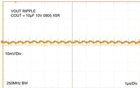
Figure 15. Output Ripple  $V_{OUT} = 1.2\text{ V}$
