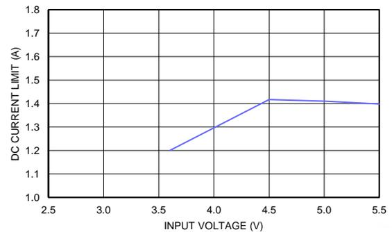
Figure 36. DC Current Limit  $V_{OUT} = 3.3\text{ V}$ ,  $T_A = 85^\circ\text{C}$
