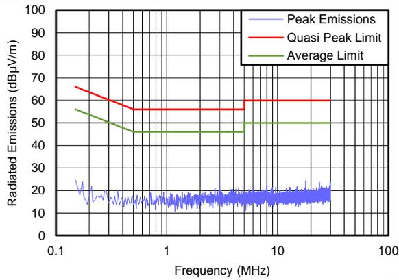
**Figure 7. Conducted EMI  $V_{IN} = 5.0\text{ V}$ ,  $V_{OUT} = 1.8\text{ V}$ ,  $I_{OUT} = 1\text{-A}$  Default Evaluation Board BOM with Additional 2.2-µH 1-µF LC Input Filter**
