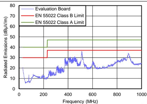
**Figure 6. Radiated EMI (Cispr22)  $V_{IN} = 5\text{ V}$ ,  $V_{OUT} = 1.8\text{ V}$ ,  $I_{OUT} = 1\text{-A}$  Default Evaluation Board BOM**
