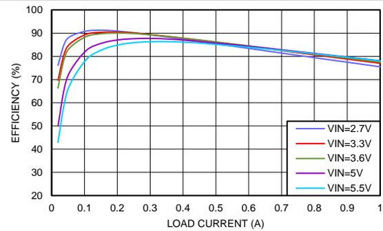
Figure 14. Efficiency  $V_{OUT} = 1.2\text{ V}$
