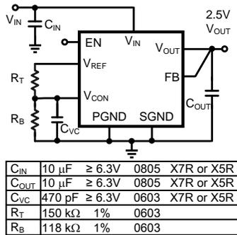
Figure 25. Schematic  $V_{OUT} = 2.5 V$
