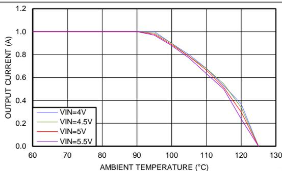
**Figure 5. Thermal Derating  $V_{OUT} = 3.3\text{ V}$ ,  $\Theta_{JA} = 77^\circ\text{C/W}$**
