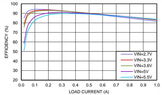
Figure 20. Efficiency  $V_{OUT} = 1.8\text{ V}$
