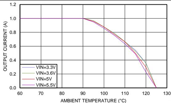
**Figure 4. Thermal Derating  $V_{OUT} = 2.5\text{ V}$ ,  $\Theta_{JA} = 77^\circ\text{C/W}$**
