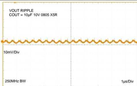
Figure 33. Output Ripple  $V_{OUT} = 3.3\text{ V}$
