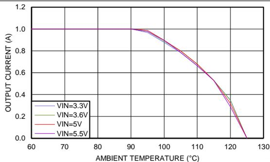
**Figure 2. Thermal Derating  $V_{OUT} = 1.2\text{ V}$ ,  $\Theta_{JA} = 77^\circ\text{C/W}$**
