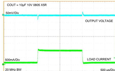
Figure 16. Load Transient  $V_{OUT} = 1.2\text{ V}$
