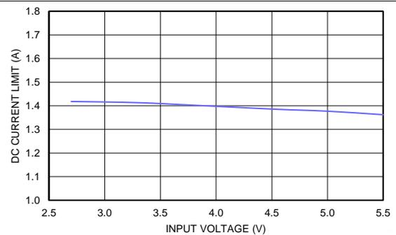
Figure 24. DC Current Limit  $V_{OUT} = 1.8\text{ V}$ ,  $T_A = 85^\circ\text{C}$
