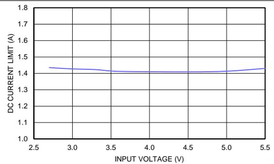
Figure 18. DC Current Limit  $V_{OUT} = 1.2\text{ V}$ ,  $T_A=85^\circ\text{C}$
