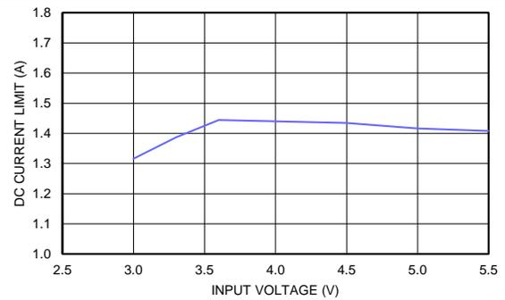
Figure 30. DC Current Limit  $V_{OUT} = 2.5 V, T_A = 85^\circ C$
