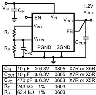
Figure 13. Schematic  $V_{OUT} = 1.2\text{ V}$
