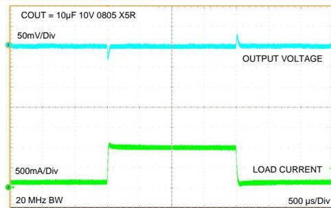
Figure 28. Load Transient  $V_{OUT} = 2.5 V$
