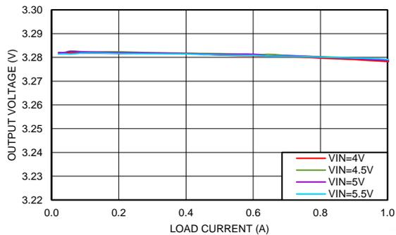
Figure 35. Line and Load Regulation  $V_{OUT} = 3.3\text{ V}$
