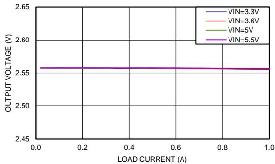
Figure 29. Line and Load Regulation  $V_{OUT} = 2.5 V$
