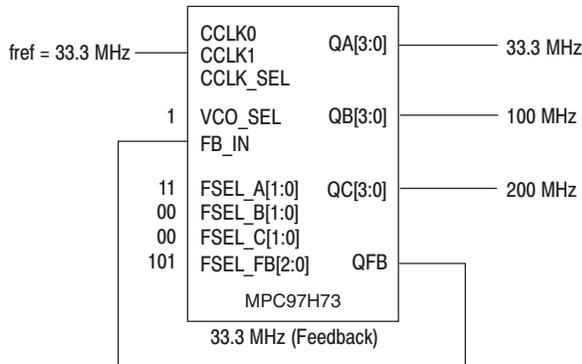
MPC97H73 example configuration (feedback of QFB = 33.3 MHz,  $f_{VCO}$ =400 MHz,  $VCO\_SEL$ =+1,  $M$ =12,  $N_A$ =12,  $N_B$ =4,  $N_C$ =2).
