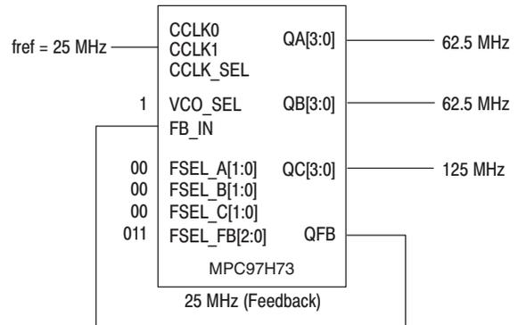
MPC97H73 example configuration (feedback of QFB = 25 MHz,  $f_{VCO}$ =250 MHz,  $VCO\_SEL$ =+1,  $M$ =10,  $N_A$ =4,  $N_B$ =4,  $N_C$ =2).
