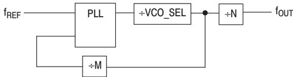
where  $f_{REF}$  is the reference frequency of the selected input clock source (CCLK0, CCLK1 or PCLK), M is the PLL feedback divider and N is a output divider. The PLL feedback divider is configured by the FSEL\_FB[2:0] and the output dividers are individually configured for each output bank by the FSEL\_A[1:0], FSEL\_B[1:0] and FSEL\_C[1:0] inputs.
