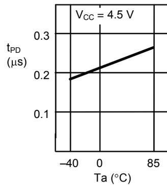
2.7 Data output delay time  $t_{PD}$
