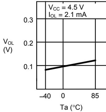
1. 22 Low-level output voltage  $V_{OL}$
