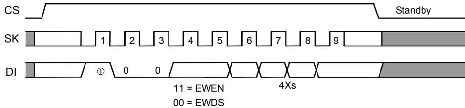
**Figure 18 Write Enable / Disable Timing (S-93C46B)**
