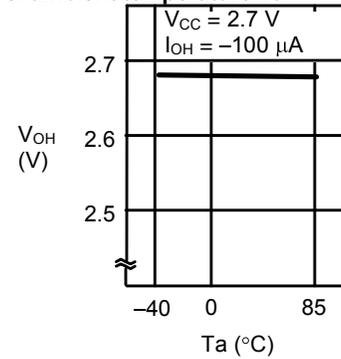
1. 19 High-level output voltage  $V_{OH}$
