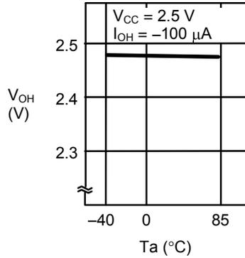
1. 20 High-level output voltage  $V_{OH}$
