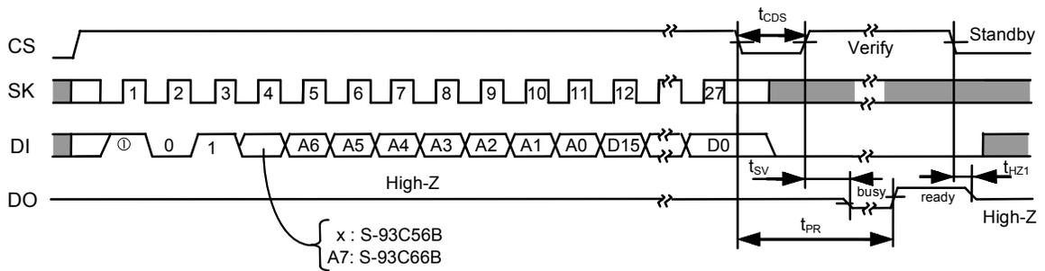
**Figure 11 Data Write Timing (S-93C56B, S-93C66B)**
