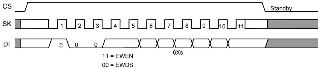
**Figure 19 Write Enable / Disable Timing (S-93C56B, S-93C66B)**
