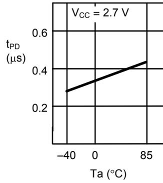
2.8 Data output delay time  $t_{PD}$
