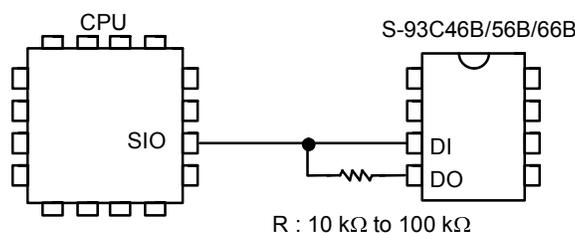
Figure 22 Connection of 3-Wire Interface
