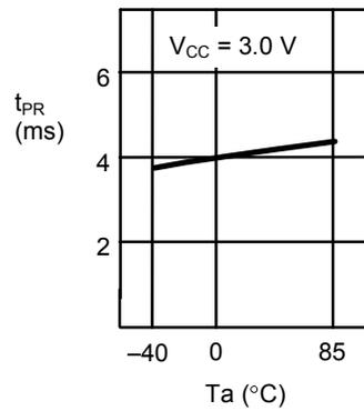
**2.5 Write time  $t_{PR}$  vs. ambient temperature  $T_a$**
