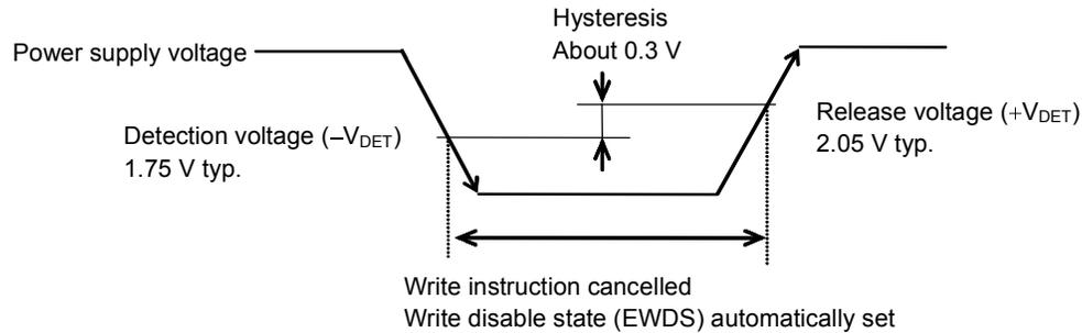
**Figure 20** Operation during Low Power Supply Voltage
