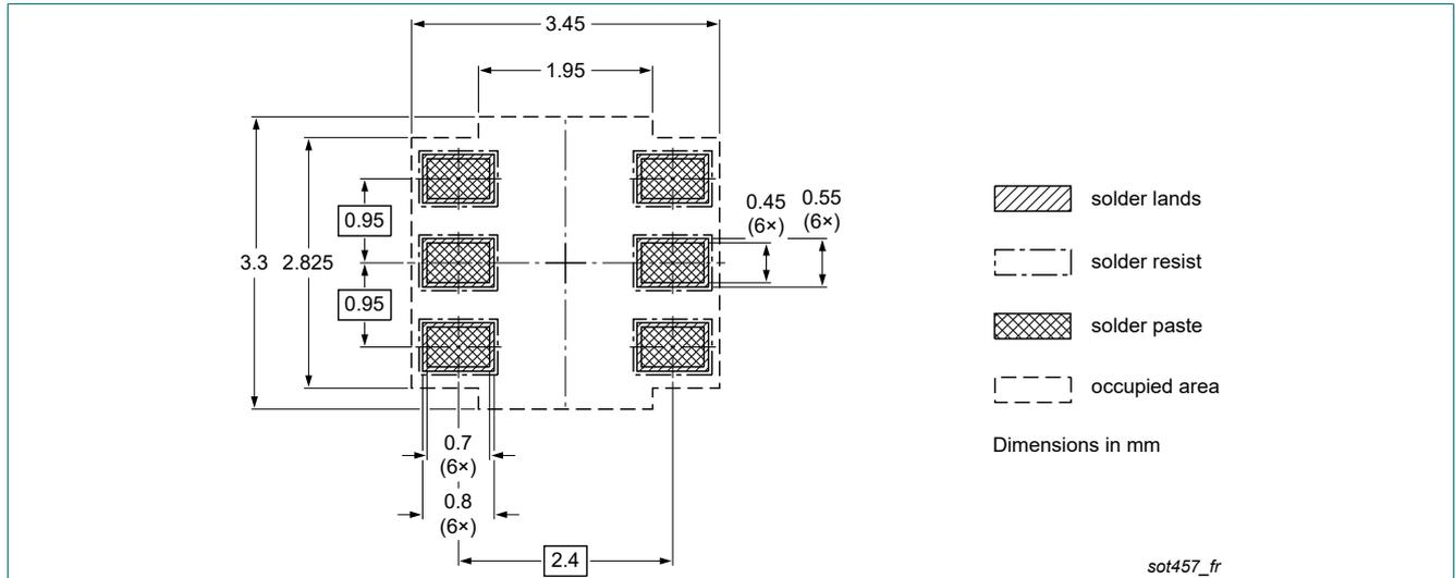
Fig. 19. Reflow soldering footprint for SC-74; TSOP6 (SOT457)
