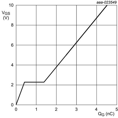
$V_{DS} = 50\text{ V}; I_D = 1.5\text{ A}$
