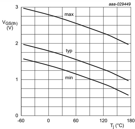
$$I_D = 250 \mu A; V_{DS} = V_{GS}$$
