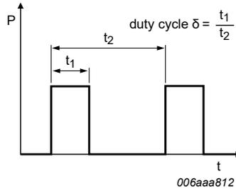
Fig. 17. Duty cycle definition
