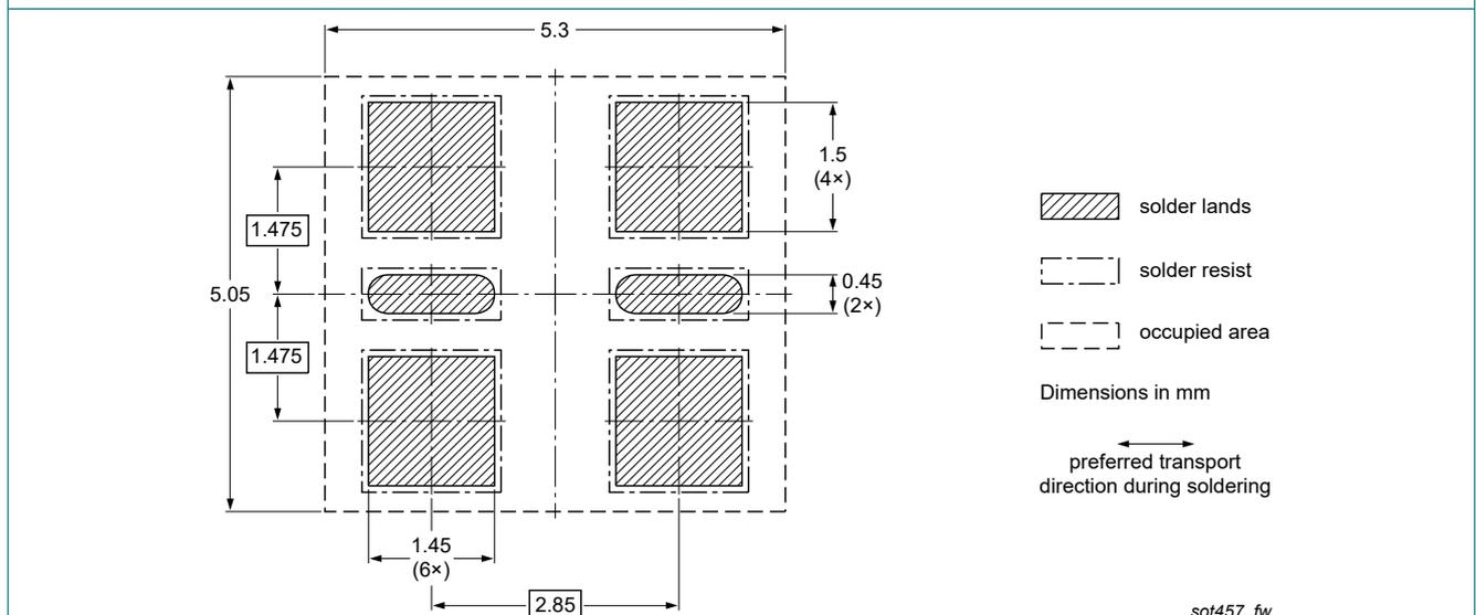
Fig. 20. Wave soldering footprint for SC-74; TSOP6 (SOT457)
