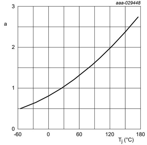
$$a = \frac{R_{DSon}}{R_{DSon}(25^\circ C)}$$
