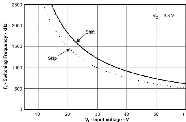
**Figure 42. Maximum Switching Frequency vs. Input Voltage**
