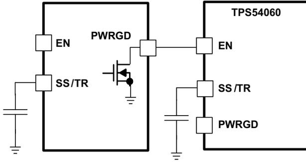
Figure 32. Schematic for Sequential Start-Up Sequence
