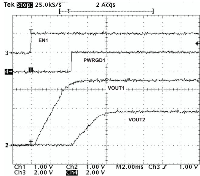
Figure 33. Sequential Startup using EN and PWRGD
