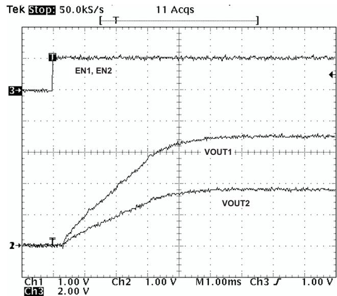
Figure 35. Ratio-Metric Startup using Coupled SS/TR pins
