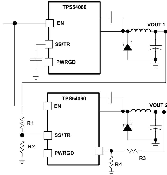
**Figure 36. Schematic for Ratiometric and Simultaneous Start-Up Sequence**
