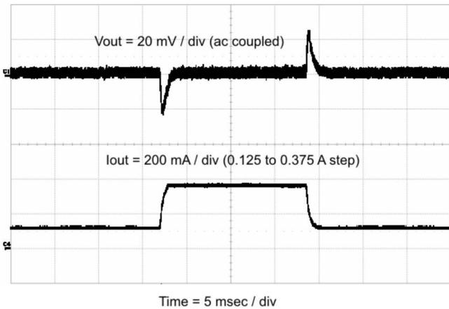
Figure 52. Load Transient
