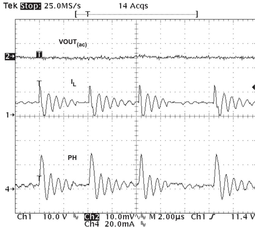
**Figure 25. Pulse Skip Mode Operation****Low Dropout Operation and Bootstrap Voltage (BOOT)**
