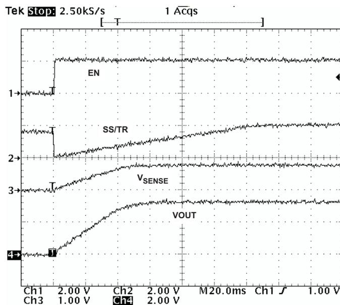
**Figure 31. Operation of SS/TR Pin when Starting**
