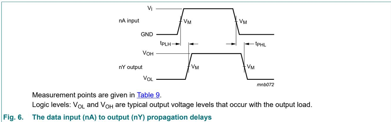
**Fig. 6. The data input (nA) to output (nY) propagation delays**
