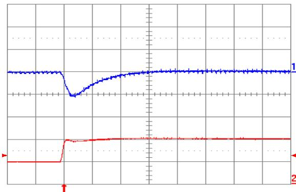
Fig. 1.0V.7: Output voltage response for  $V_{out} = 1.0V$  to positive load current step change from 5A to 10A with slew rate of  $5A/\mu s$  at  $V_{in} = 12V$ . Top trace: output voltage (100mV/div.); Bottom trace: load current (5A/div.).  $C_o = 100\mu F$  ceramic. Time scale:  $20\mu s$ /div.
