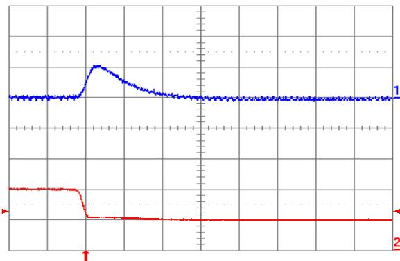
Fig. 1.0V.8: Output voltage response for  $V_{out} = 1.0V$  to negative load current step change from 10A to 5A with slew rate of  $-5A/\mu s$  at  $V_{in} = 12V$ . Top trace: output voltage (100mV/div.); Bottom trace: load current (5A/div.).  $C_o = 100\mu F$  ceramic. Time scale:  $20\mu s$ /div.
