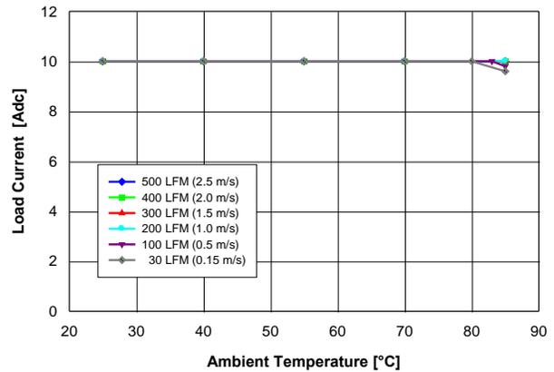
Fig. 1.8V.2: Available load current vs. ambient temperature and airflow rates for  $V_{out} = 1.8V$  converter mounted horizontally with  $V_{in} = 12V$ , and maximum MOSFET temperature  $\leq 120^\circ C$ .
