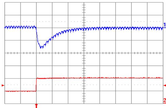
Fig. 3.3V.7: Output voltage response for  $V_{out} = 3.3V$  to positive load current step change from 5A to 10A with slew rate of  $5A/\mu s$  at  $V_{in} = 12V$ . Top trace: output voltage (100mV/div.); Bottom trace: load current (5A/div.).  $C_o = 100\mu F$  ceramic. Time scale:  $20\mu s$ /div.
