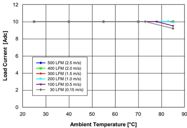
Fig. 3.3V.1: Available load current vs. ambient temperature and airflow rates for  $V_{out} = 3.3V$  converter mounted vertically with  $V_{in} = 12V$ , and maximum MOSFET temperature  $\leq 120^\circ C$ .
