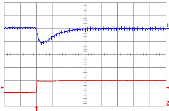
Fig. 1.5V.7: Output voltage response for  $V_{out} = 1.5V$  to positive load current step change from 5A to 10A with slew rate of  $5A/\mu s$  at  $V_{in} = 12V$ . Top trace: output voltage (100mV/div.); Bottom trace: load current (5A/div.);  $C_o = 100\mu F$  ceramic. Time scale: 20µs/div.
