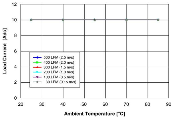
Fig. 1.0V.1: Available load current vs. ambient temperature and airflow rates for  $V_{out} = 1.0V$  converter mounted vertically with  $V_{in} = 12V$ , and maximum MOSFET temperature  $\leq 120^\circ C$ .
