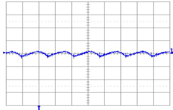
Fig. 2.0V.6: Output voltage ripple (20mV/div.) at full rated load current into a resistive load with external capacitance  $100\mu F$  ceramic and  $V_{in} = 12V$  for  $V_{out} = 2.0V$ . Time scale: 2µs/div.
