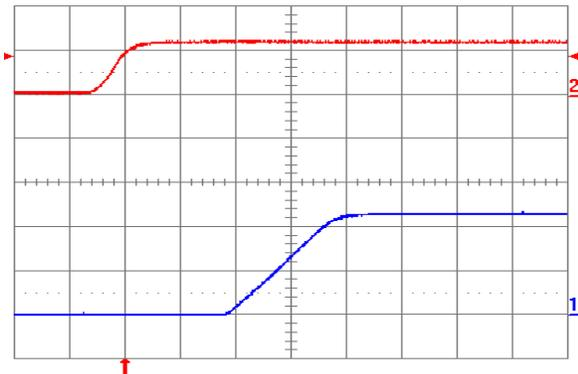
Fig. 1.2V.5: Turn-on transient for  $V_{out} = 1.2V$  with application of  $V_{in}$  at full rated load current (resistive) and  $100\mu F$  external capacitance at  $V_{in} = 12V$ . Top trace:  $V_{in}$  (10V/div.); Bottom trace: output voltage (0.5V/div.); Time scale: 2ms/div.
