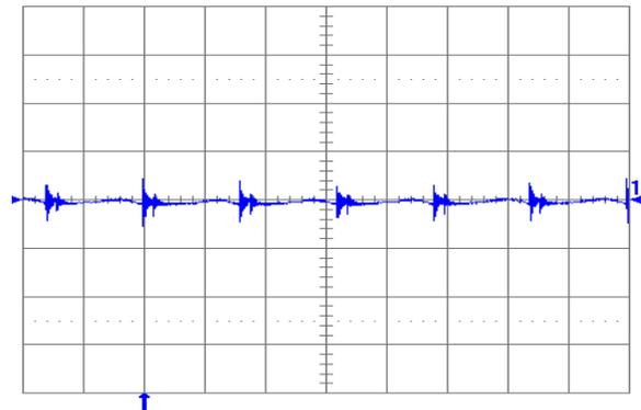
Fig. 1.2V.6: Output voltage ripple (20mV/div.) at full rated load current into a resistive load with external capacitance  $100\mu F$  ceramic and  $V_{in} = 12V$  for  $V_{out} = 1.2V$ . Time scale: 2µs/div.
