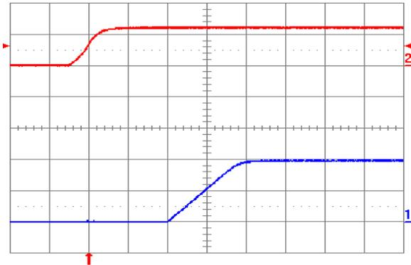
Fig. 1.0V.5: Turn-on transient for  $V_{out} = 1.0V$  with application of  $V_{in}$  at full rated load current (resistive) and  $100\mu F$  external capacitance at  $V_{in} = 12V$ . Top trace:  $V_{in}$  (10V/div.); Bottom trace: output voltage (0.5V/div.); Time scale: 2ms/div.
