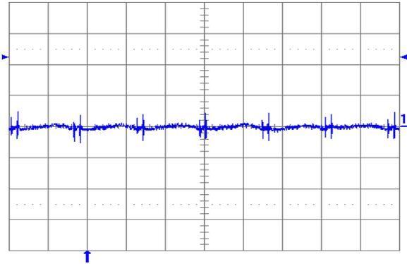
Fig. 1.0V.6: Output voltage ripple (20mV/div.) at full rated load current into a resistive load with external capacitance  $100\mu F$  ceramic and  $V_{in} = 12V$  for  $V_{out} = 1.0V$ . Time scale:  $2\mu s$ /div.
