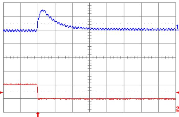
Fig. 3.3V.8: Output voltage response for  $V_{out} = 3.3V$  to negative load current step change from 10A to 5A with slew rate of  $-5A/\mu s$  at  $V_{in} = 12V$ . Top trace: output voltage (100mV/div.); Bottom trace: load current (5A/div.).  $C_o = 100\mu F$  ceramic. Time scale:  $20\mu s$ /div.
