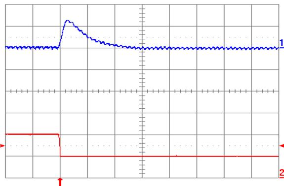
Fig. 2.5V.8: Output voltage response for  $V_{out} = 2.5V$  to negative load current step change from 10A to 5A with slew rate of  $-5A/\mu s$  at  $V_{in} = 12V$ . Top trace: output voltage (100mV/div.); Bottom trace: load current (5A/div.).  $C_o = 100\mu F$  ceramic. Time scale: 20μs/div.
