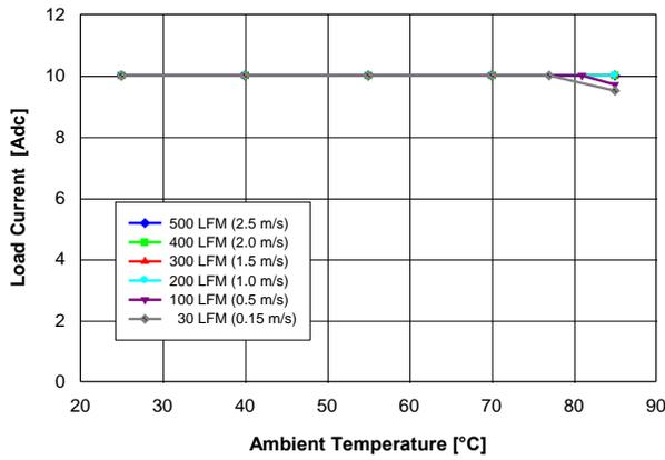
Fig. 2.0V.1: Available load current vs. ambient temperature and airflow rates for  $V_{out} = 2.0V$  converter mounted vertically with  $V_{in} = 12V$ , and maximum MOSFET temperature  $\leq 120^{\circ}C$ .
