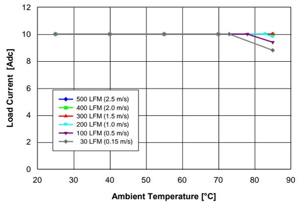
Fig. 3.3V.2: Available load current vs. ambient temperature and airflow rates for  $V_{out} = 3.3V$  converter mounted horizontally with  $V_{in} = 12V$ , and maximum MOSFET temperature  $\leq 120^\circ C$ .
