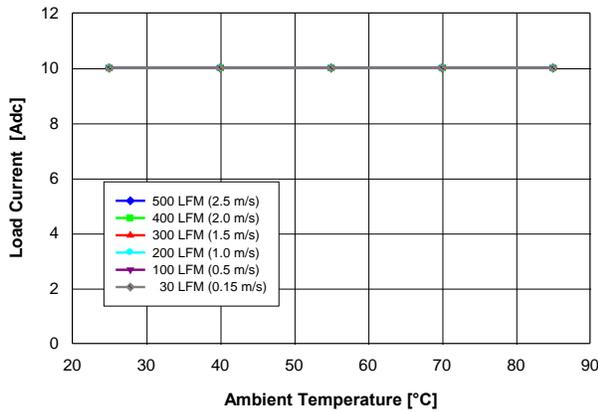
Fig. 1.2V.1: Available load current vs. ambient temperature and airflow rates for  $V_{out} = 1.2V$  converter mounted vertically with  $V_{in} = 12V$ , and maximum MOSFET temperature  $\leq 120^{\circ}C$ .
