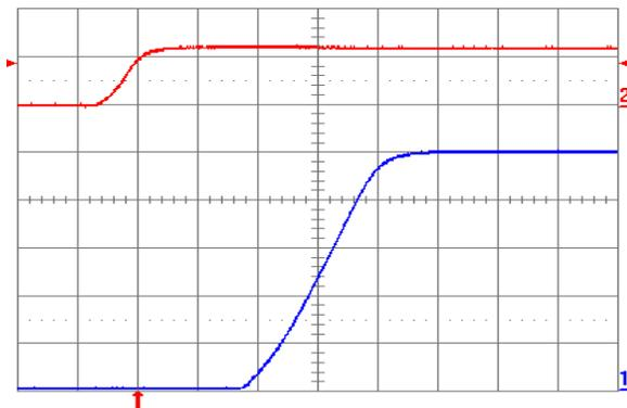
Fig. 5.0V.5: Turn-on transient for  $V_{out} = 5.0V$  with application of  $V_{in}$  at full rated load current (resistive) and  $100\mu F$  external capacitance at  $V_{in} = 12V$ . Top trace:  $V_{in}$  (10V/div.); Bottom trace: output voltage (1V/div.); Time scale: 2ms/div.
