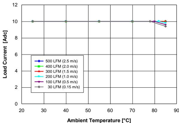
Fig. 2.5V.1: Available load current vs. ambient temperature and airflow rates for  $V_{out} = 2.5V$  converter mounted vertically with  $V_{in} = 12V$ , and maximum MOSFET temperature  $\leq 120^\circ C$ .
