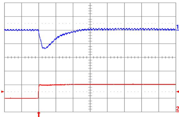
Fig. 2.5V.7: Output voltage response for  $V_{out} = 2.5V$  to positive load current step change from 5A to 10A with slew rate of  $5A/\mu s$  at  $V_{in} = 12V$ . Top trace: output voltage (100mV/div.); Bottom trace: load current (5A/div.).  $C_o = 100\mu F$  ceramic. Time scale: 20μs/div.
