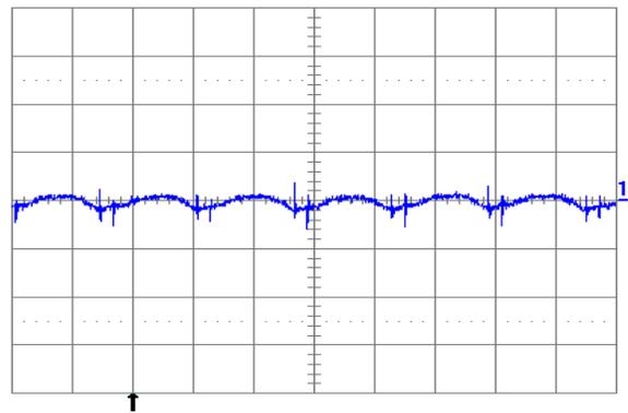
Fig. 1.5V.6: Output voltage ripple (20mV/div.) at full rated load current into a resistive load with external capacitance  $100\mu F$  ceramic and  $V_{in} = 12V$  for  $V_{out} = 1.5V$ . Time scale: 2µs/div.
