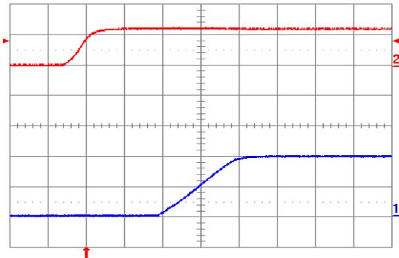
Fig. 2.0V.5: Turn-on transient for  $V_{out} = 2.0V$  with application of  $V_{in}$  at full rated load current (resistive) and  $100\mu F$  external capacitance at  $V_{in} = 12V$ . Top trace:  $V_{in}$  (10V/div.); Bottom trace: output voltage (1V/div.); Time scale: 2ms/div.
