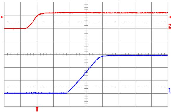
Fig. 1.5V.5: Turn-on transient for  $V_{out} = 1.5V$  with application of  $V_{in}$  at full rated load current (resistive) and  $100\mu F$  external capacitance at  $V_{in} = 12V$ . Top trace:  $V_{in}$  (10V/div.); Bottom trace: output voltage (0.5V/div.); Time scale: 2ms/div.
