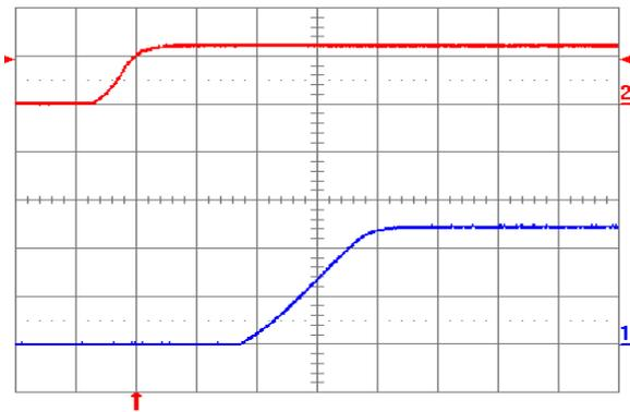
Fig. 2.5V.5: Turn-on transient for  $V_{out} = 2.5V$  with application of  $V_{in}$  at full rated load current (resistive) and  $100\mu F$  external capacitance at  $V_{in} = 12V$ . Top trace:  $V_{in}$  (10V/div.); Bottom trace: output voltage (1V/div.); Time scale: 2ms/div.
