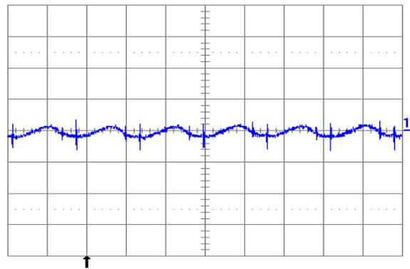
Fig. 2.5V.6: Output voltage ripple (20mV/div.) at full rated load current into a resistive load with external capacitance  $100\mu F$  ceramic and  $V_{in} = 12V$  for  $V_{out} = 2.5V$ . Time scale: 2μs/div.
