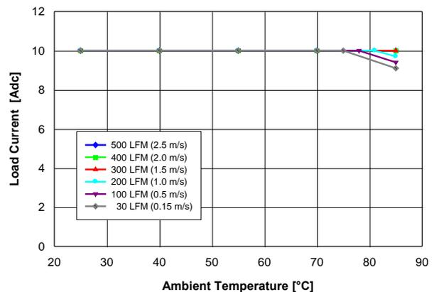
Fig. 2.5V.2: Available load current vs. ambient temperature and airflow rates for  $V_{out} = 2.5V$  converter mounted horizontally with  $V_{in} = 12V$ , and maximum MOSFET temperature  $\leq 120^\circ C$ .
