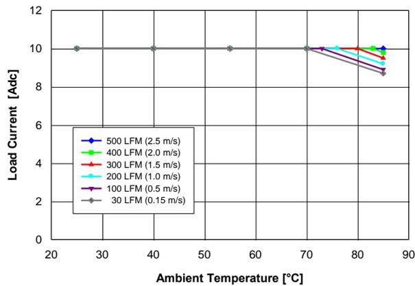
Fig. 5.0V.1: Available load current vs. ambient temperature and airflow rates for  $V_{out} = 5.0V$  converter mounted vertically with  $V_{in} = 12V$ , and maximum MOSFET temperature  $\leq 120^{\circ}C$ .
