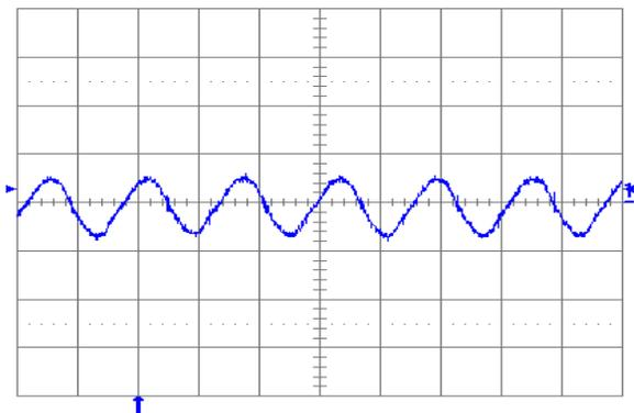
Fig. 5.0V.6: Output voltage ripple (20mV/div.) at full rated load current into a resistive load with external capacitance  $100\mu F$  ceramic and  $V_{in} = 12V$  for  $V_{out} = 5.0V$ . Time scale: 2µs/div.
