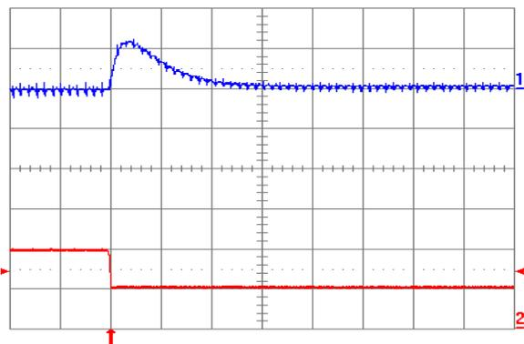
Fig. 1.5V.8: Output voltage response for  $V_{out} = 1.5V$  to negative load current step change from 10A to 5A with slew rate of  $-5A/\mu s$  at  $V_{in} = 12V$ . Top trace: output voltage (100mV/div.); Bottom trace: load current (5A/div.);  $C_o = 100\mu F$  ceramic. Time scale: 20µs/div.
