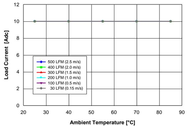
Fig. 1.0V.2: Available load current vs. ambient temperature and airflow rates for  $V_{out} = 1.0V$  converter mounted horizontally with  $V_{in} = 12V$ , and maximum MOSFET temperature  $\leq 120^\circ C$ .
