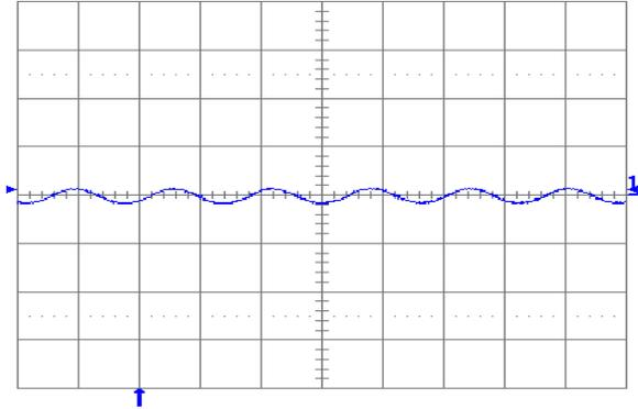
Fig. 1.8V.6: Output voltage ripple (20mV/div.) at full rated load current into a resistive load with external capacitance  $100\mu F$  ceramic and  $V_{in} = 12V$  for  $V_{out} = 1.8V$ . Time scale:  $2\mu s$ /div.
