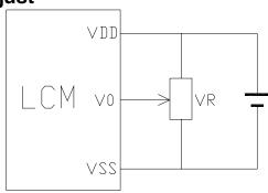
VDD~V0: LCD Driving voltage
