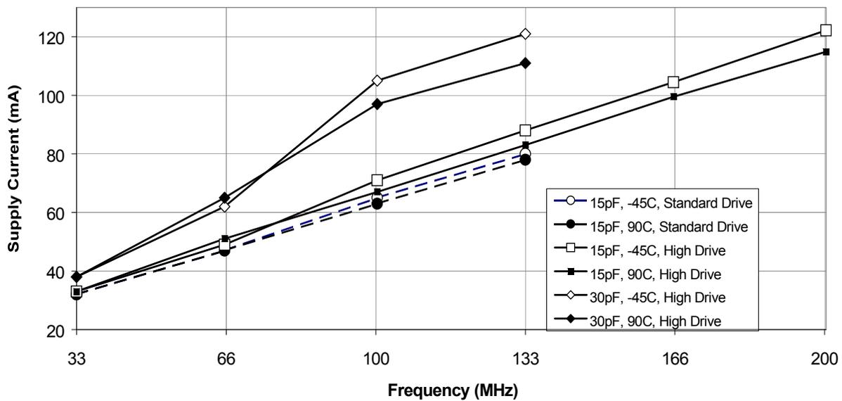
Note that the 30-pF high-drive data above 100MHz is beyond the data sheet specification of 22 pF.
