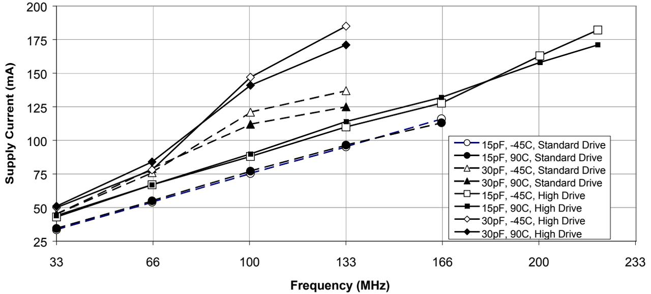
Note that the 30-pF data above 100 MHz is beyond the data sheet specification of 22 pF.
