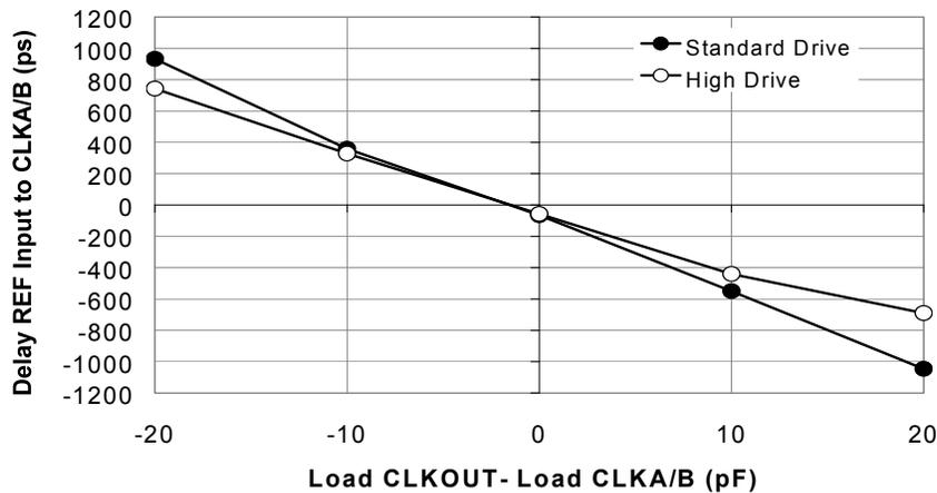
Data is shown for 66 MHz. Delay is a weak function of frequency.
