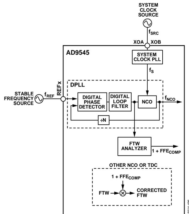
Figure 103. Closed-Loop Method
