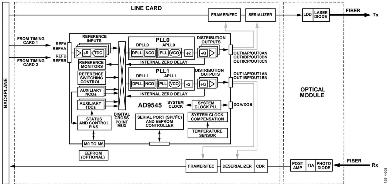
Figure 115. Optical Line Card Direct Timing Example
