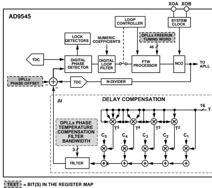
Figure 83. Delay Compensation
