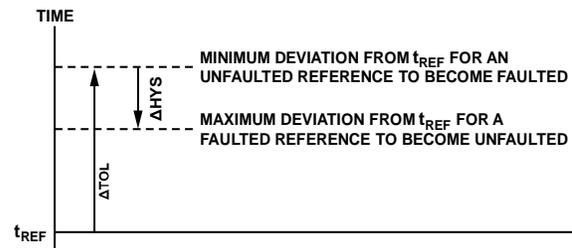
Figure 50. Reference Monitor Fault and Unfault Parameters
