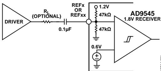
Figure 32. Single-Ended AC-Coupled Interface Mode
