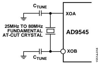
Figure 29. System Clock Input (XOA/XOB) Using the Crystal Path
