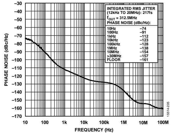
Figure 7. Absolute Phase Noise (PLL0, Configuration 5, HCSL Mode,  $f_{REF} = 25\text{ MHz}$ ,  $f_{OUT} = 312.5\text{ MHz}$ ,  $f_{OSC} = 52\text{ MHz}$  Crystal,  $50\text{ Hz}$  DPLL BW, Phase Buildout Mode)
