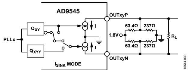
Figure 41. LVDS-Compatible Output, 1.2 V Common-Mode, Thevenin Bias Network (I = 7.5 mA; 15 mA with Extra 100 Ω Termination, R<sub>L</sub>)
