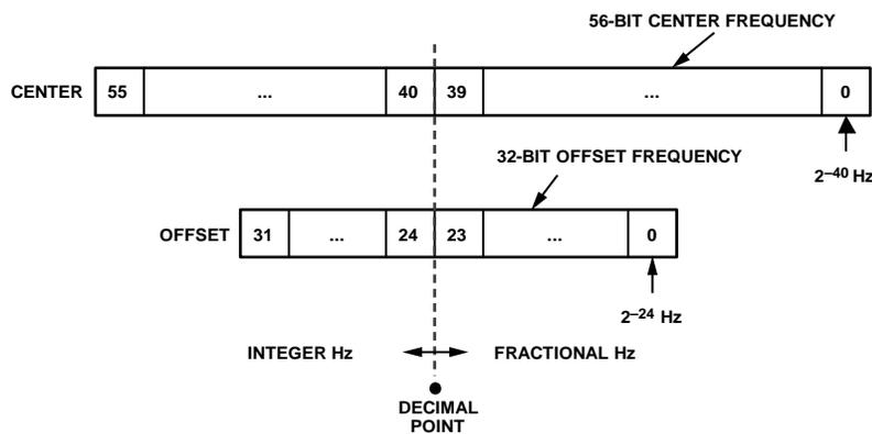
Figure 99. Auxiliary NCO Frequency Tuning
