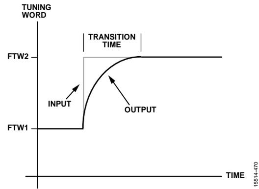
Figure 78. NCO Gain Tuning Word Filter Response
