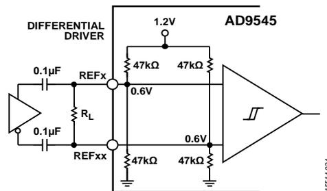
Figure 35. Differential AC-Coupled Mode
