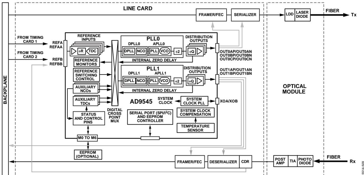
Figure 116. Optical Line Card Loop Timing Example
