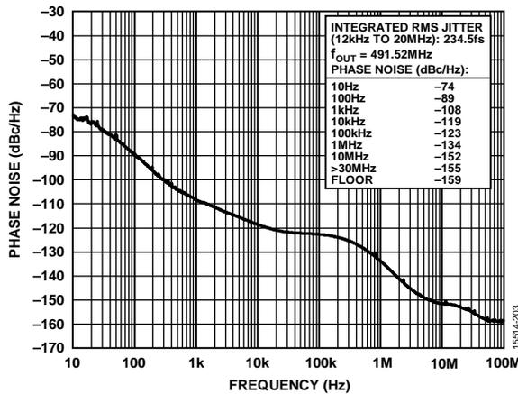
Figure 5. Absolute Phase Noise (PLL0, Configuration 3, HCSL Mode,  $f_{REF} = 1\text{ Hz}$ ,  $f_{OUT} = 491.52\text{ MHz}$ ,  $f_{COMP} = 19.2\text{ MHz}$  TCXO,  $f_{OSC} = 52\text{ MHz}$  Crystal,  $0.05\text{ Hz}$  DPLL BW)
