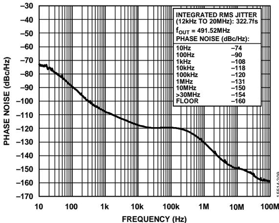
Figure 11. Absolute Phase Noise (PLL1, Configuration 3, HCSL Mode,  $f_{REF} = 1\text{ Hz}$ ,  $f_{OUT} = 491.52\text{ MHz}$ ,  $f_{COMP} = 19.2\text{ MHz}$  TCXO,  $f_{OSC} = 52\text{ MHz}$  Crystal, 0.05 Hz DPLL BW)
