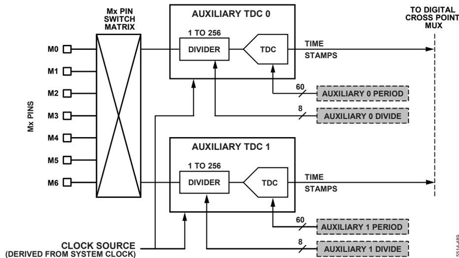
Figure 96. Auxiliary TDC Block Diagram
