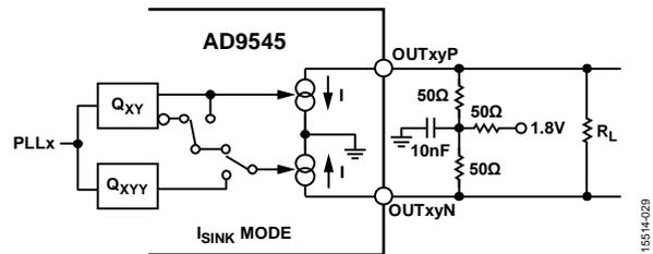
Figure 40. LVDS-Compatible Output, 1.24 V Common Mode, T Network (I = 7.5 mA; I = 15 mA with Extra 100 Ω Termination, R<sub>L</sub>)
