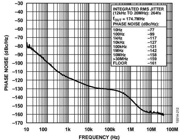
Figure 14. Absolute Phase Noise (PLL1, Configuration 6, HCSL Mode,  $f_{REF} = 155.52\text{ MHz}$ ,  $f_{OUT} = 174.7\text{ MHz}$ ,  $f_{OSC} = 52\text{ MHz}$  Crystal, 50 Hz DPLL BW, Phase Buildout Mode)
