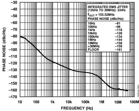
Figure 3. Absolute Phase Noise (PLL0, Configuration 1, HCSL Mode,  $f_{REF} = 38.88\text{ MHz}$ ,  $f_{OUT} = 155.52\text{ MHz}$ ,  $f_{OSC} = 52\text{ MHz}$  Crystal,  $50\text{ Hz}$  DPLL BW
