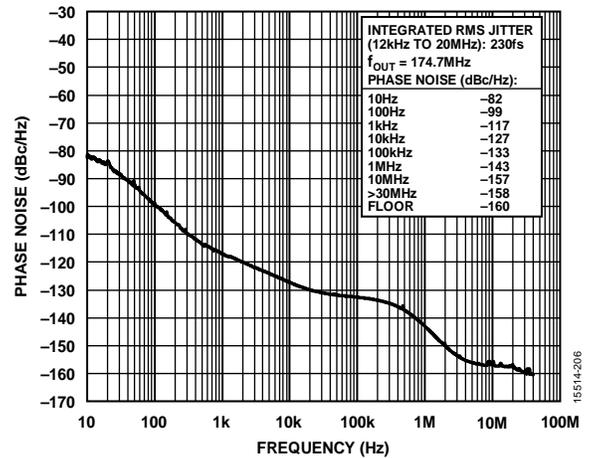
Figure 8. Absolute Phase Noise (PLL0, Configuration 6, HCSL Mode,  $f_{REF} = 155.52\text{ MHz}$ ,  $f_{OUT} = 174.7\text{ MHz}$ ,  $f_{OSC} = 52\text{ MHz}$  Crystal,  $50\text{ Hz}$  DPLL BW, Phase Buildout Mode)
