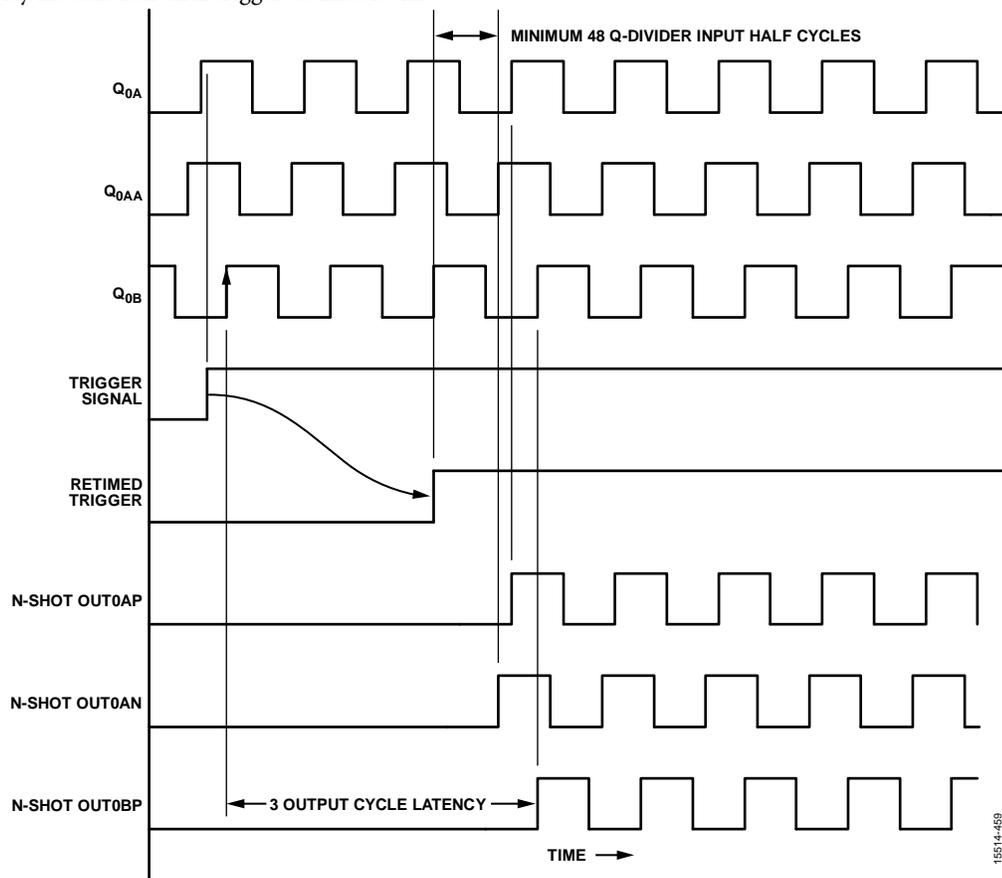
Figure 67. Trigger Retiming (with Q<sub>0AA</sub> as the Retiming Q-Divider)
