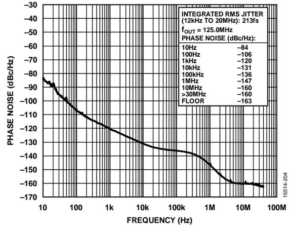
Figure 6. Absolute Phase Noise (PLL0, Configuration 4, HCSL Mode,  $f_{REF} = 125\text{ MHz}$ ,  $f_{OUT} = 125.0\text{ MHz}$ ,  $f_{COMP} = 19.2\text{ MHz}$  TCXO,  $f_{OSC} = 52\text{ MHz}$  Crystal,  $0.1\text{ Hz}$  DPLL BW, Phase Buildout Mode)
