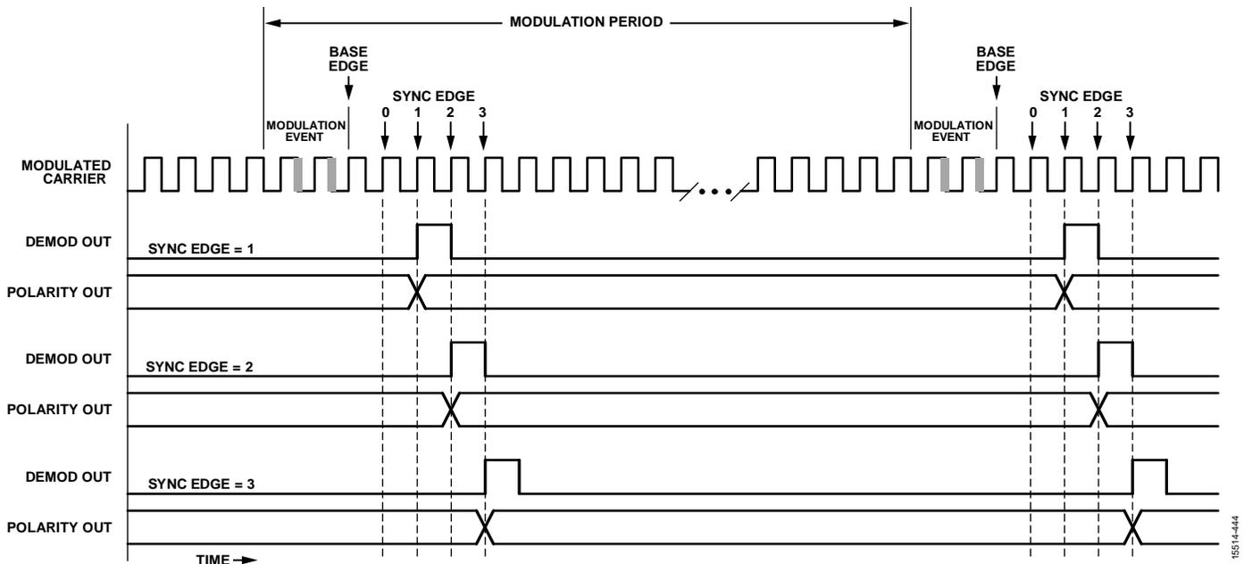
Figure 52. Demodulation Synchronization
