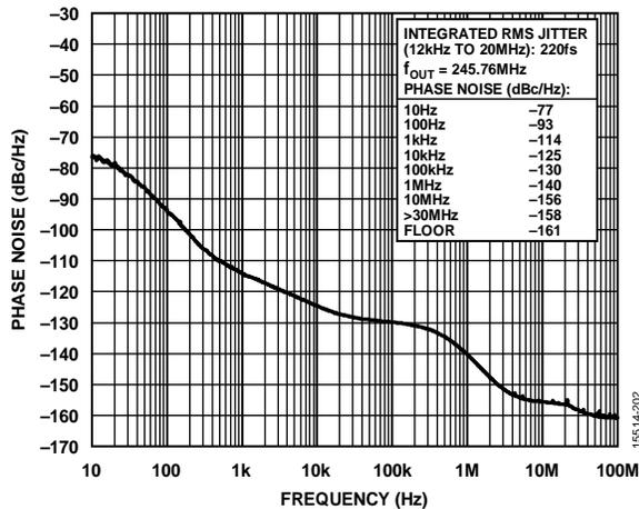
Figure 4. Absolute Phase Noise (PLL0, Configuration 2, HCSL Mode,  $f_{REF} = 30.72\text{ MHz}$ ,  $f_{OUT} = 245.76\text{ MHz}$ ,  $f_{OSC} = 52\text{ MHz}$  Crystal,  $50\text{ Hz}$  DPLL BW)
