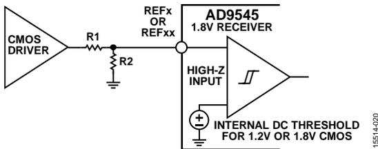
Figure 31. Single-Ended DC-Coupled Mode, 1.2 V or 1.8 V CMOS
