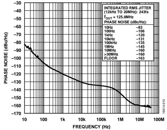
Figure 12. Absolute Phase Noise (PLL1, Configuration 4, HCSL Mode,  $f_{REF} = 125\text{ MHz}$ ,  $f_{OUT} = 125\text{ MHz}$ ,  $f_{COMP} = 19.2\text{ MHz}$  TCXO,  $f_{OSC} = 52\text{ MHz}$  Crystal, 0.1 Hz DPLL BW, Phase Buildout Mode)
