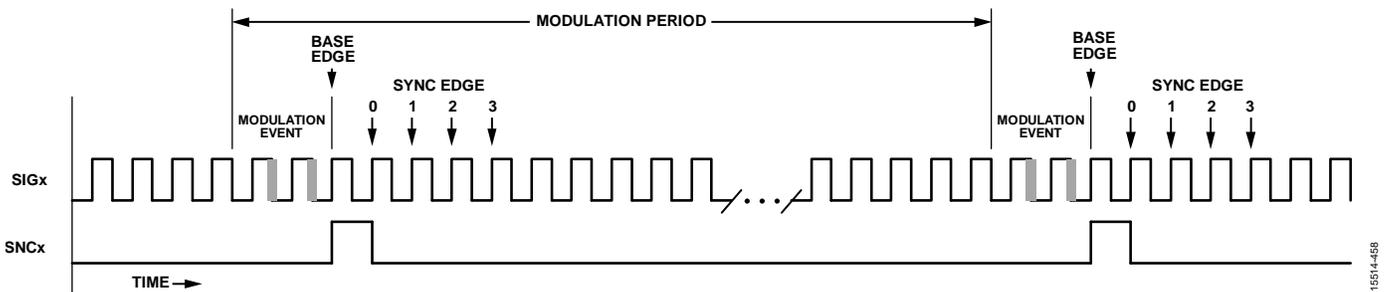
Figure 66. Modulation Synchronization
