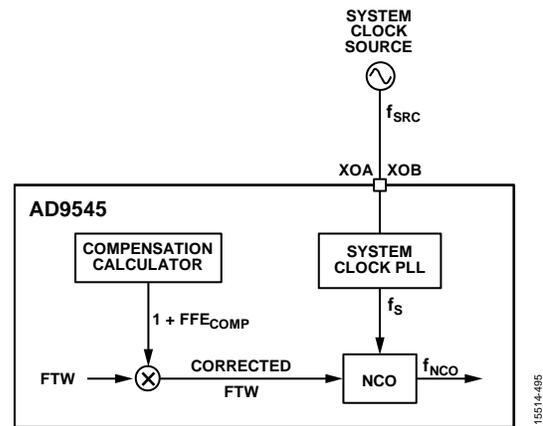
Figure 102. Open-Loop Method
