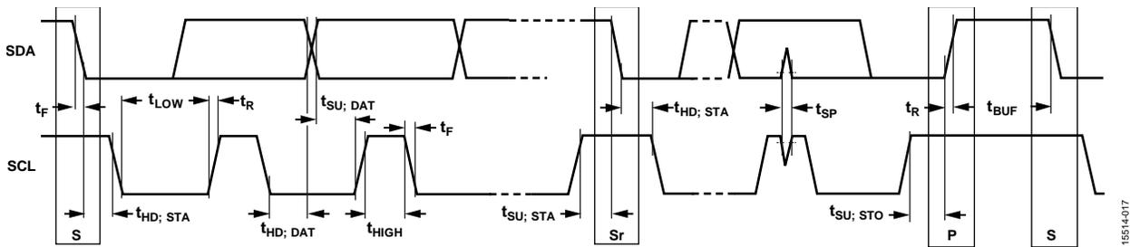
Figure 133. I<sup>2</sup>C Serial Port Timing
