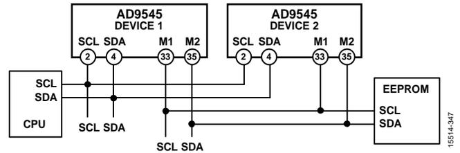
Figure 113. Level 1 Multidevice Configuration
