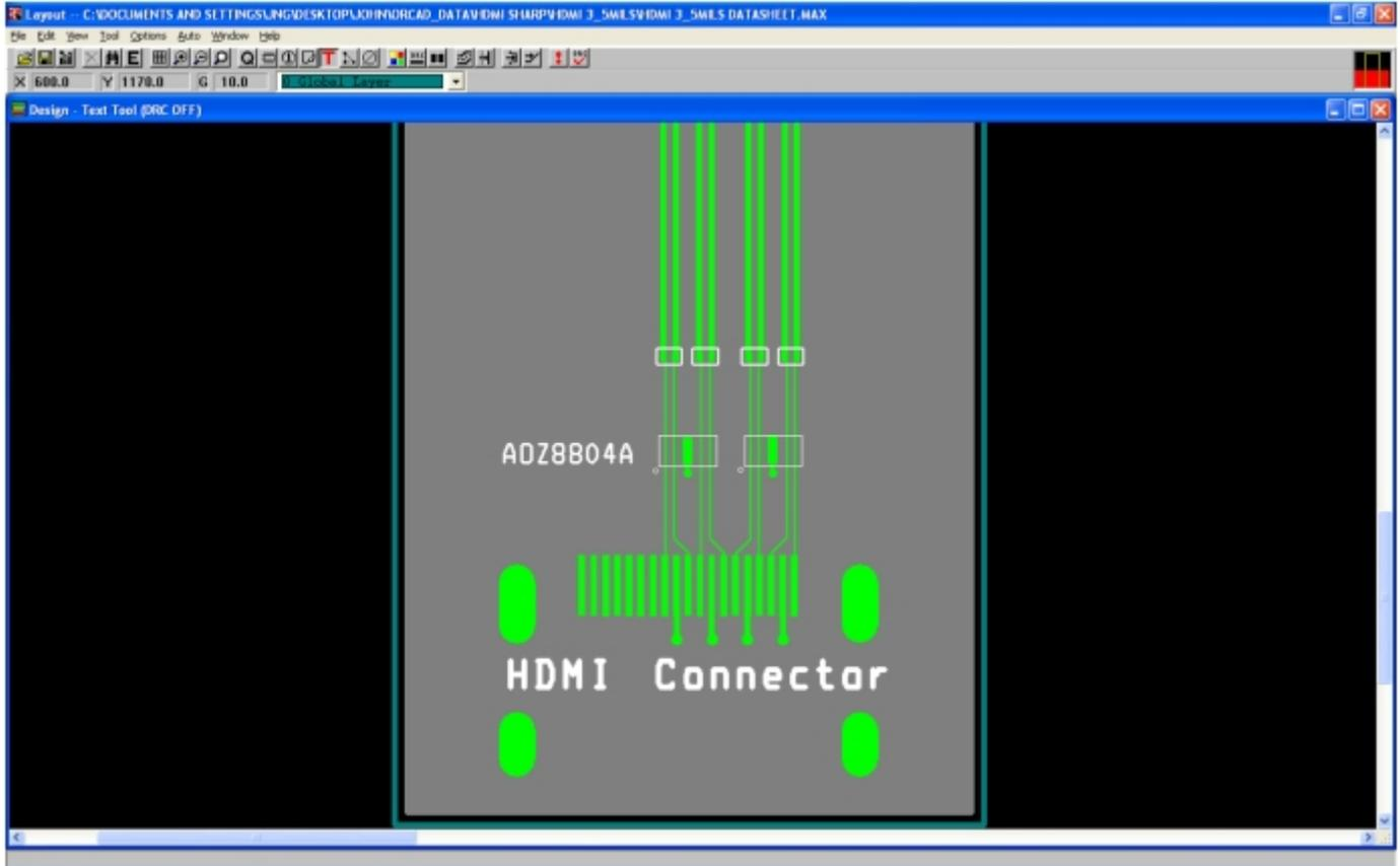
Figure 9. HDMI PCB Layout with Compensated Traces
