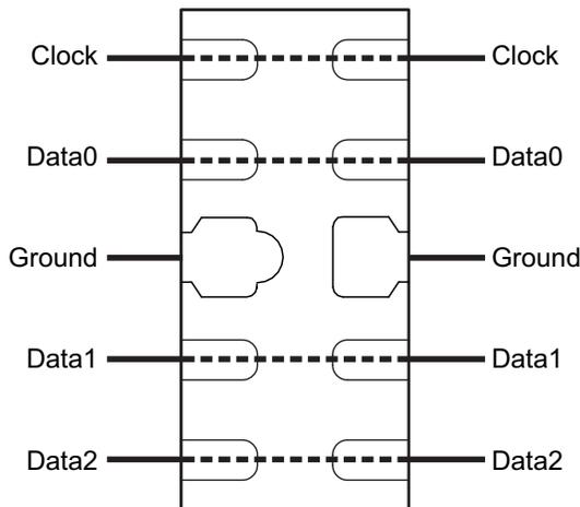
Figure 6. Flow Through Layout for HDMI
