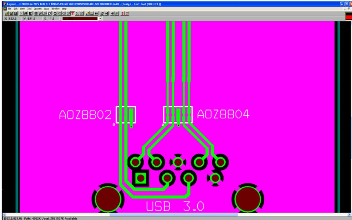
Figure 8. USB 3.0 PCB Layout with Compensated Traces
