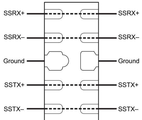
Figure 7. Flow Through Layout for USB 3.0
