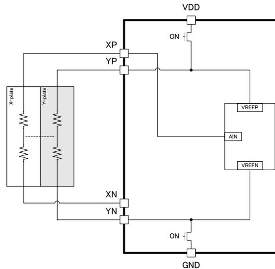
Figure 6. Y-Position Detection Mode
