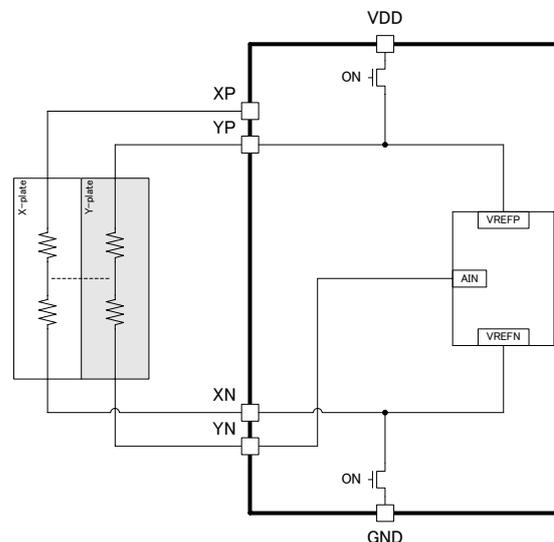
Figure 8. Z2-Position Detection Mode
