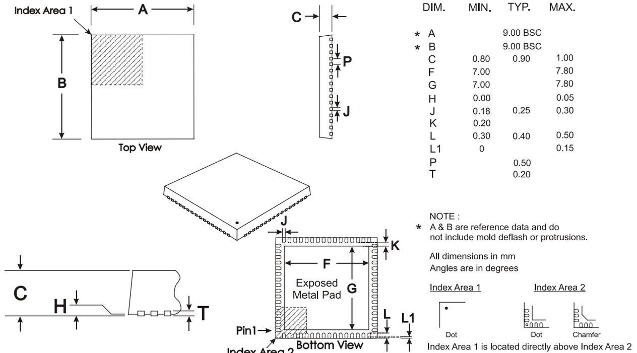
Depending on the method of lead termination at the edge of the package, pull back (L1) may be present. L minus L1 to be equal to, or greater than 0.3mm
