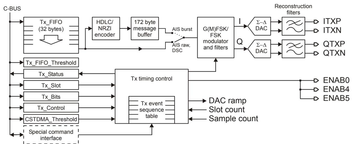
Figure 6 Transmit Channel
