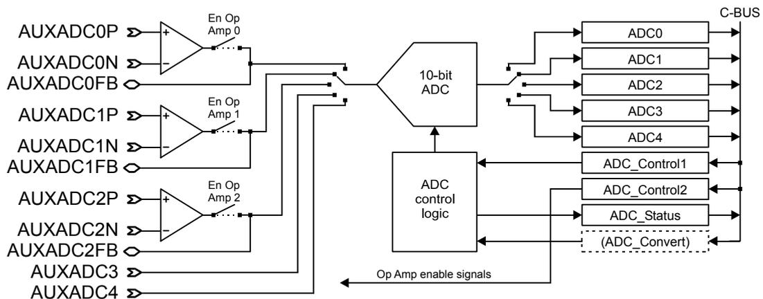
Figure 12 Auxiliary ADC
