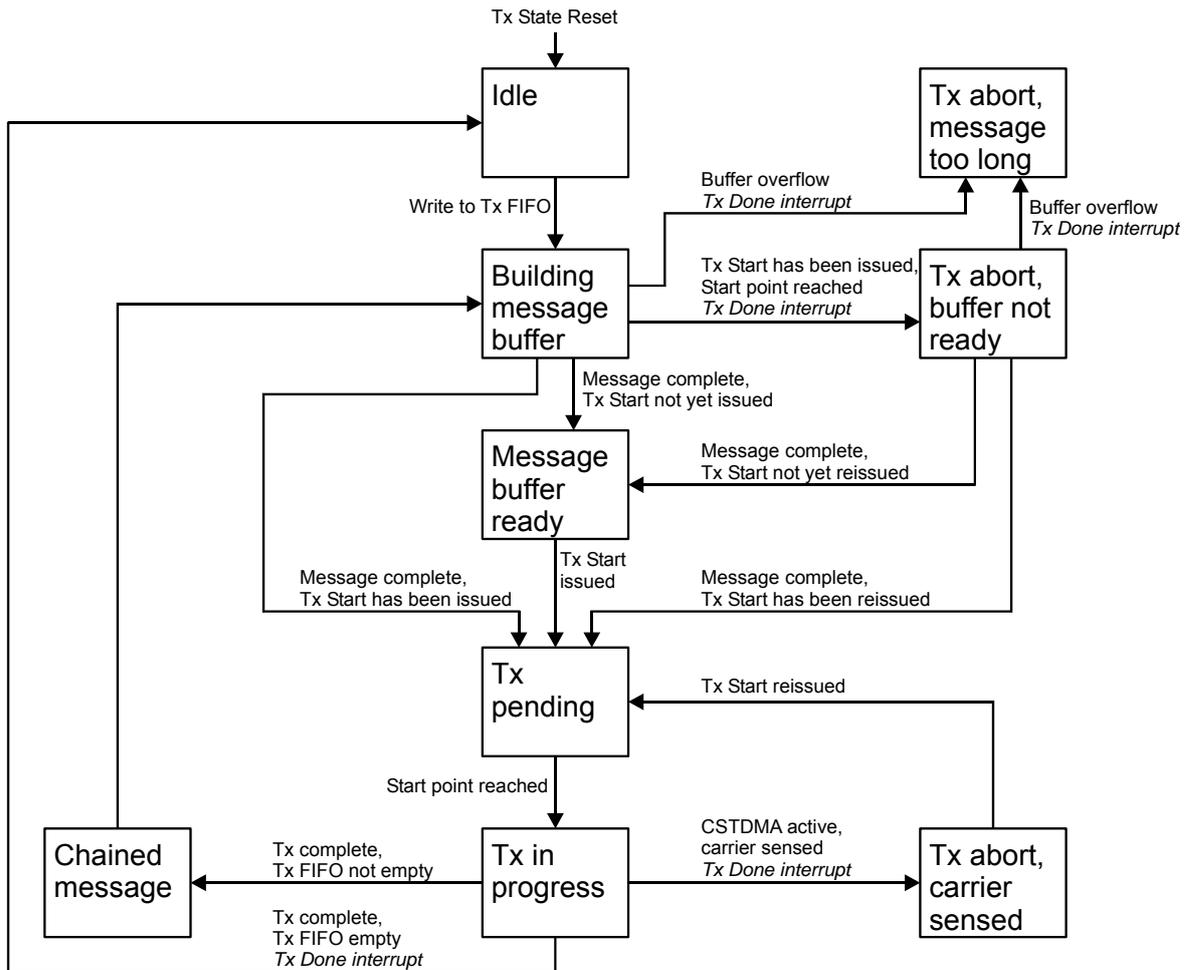
Figure 8 Tx (AIS burst mode) state transitions
