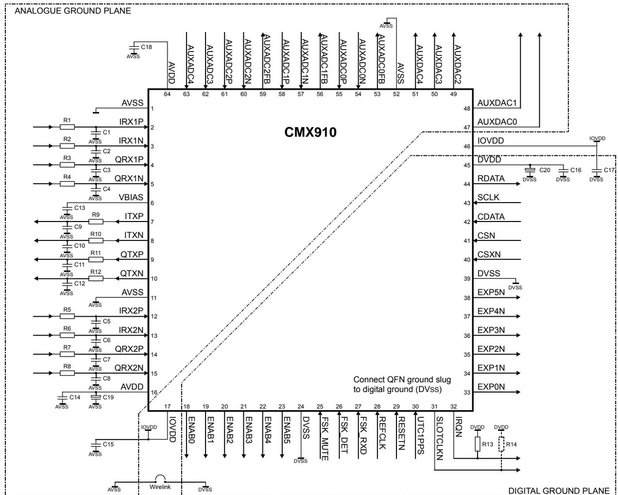
**Figure 2 Recommended External Components**
