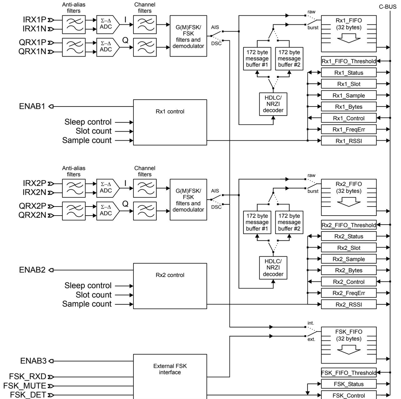
Figure 11 Receive Channel
