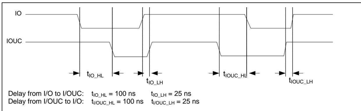
**Figure 8: I/O – I/OUC Delays: Timing Diagram**
