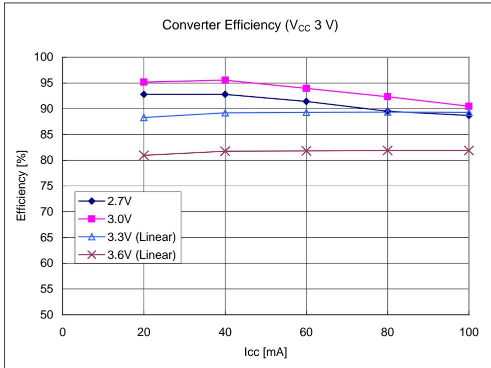
**Figure 11: DC – DC Converter Efficiency ( $V_{CC} = 3 V$ )**
