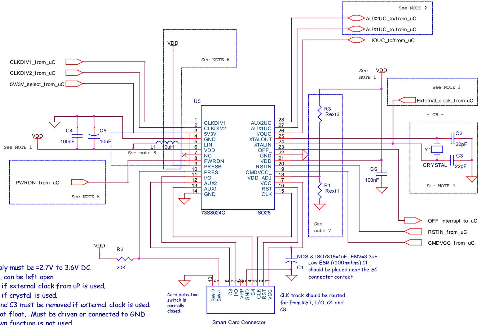
Figure 9: 73S8024C Typical Application Schematic
