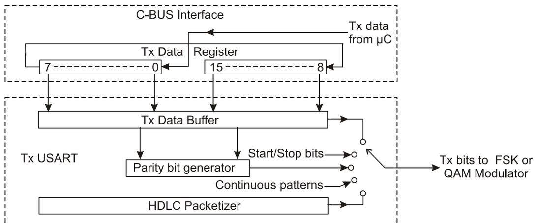
**Figure 5c Tx USART (in 16 Bit Mode)**
