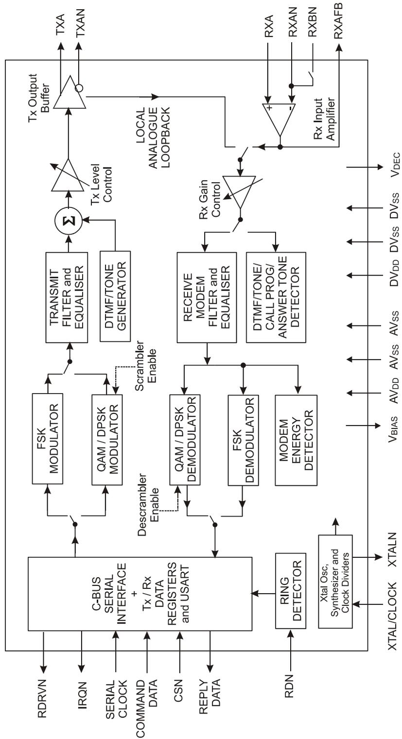
Figure 1 Block Diagram
