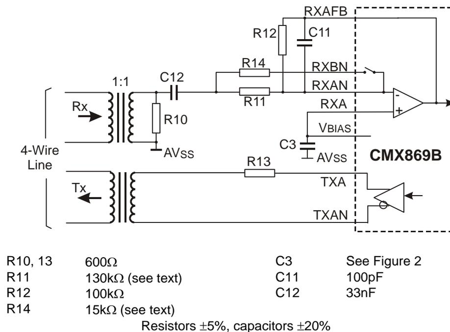
**Figure 4b 4-Wire Line Interface Circuit**
