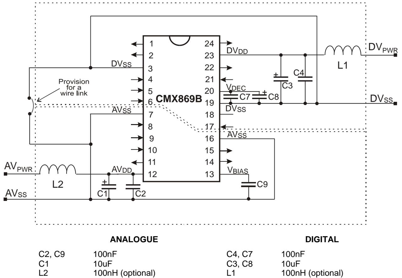
**Figure 2b Recommended Power Supply Connections and De-coupling**
