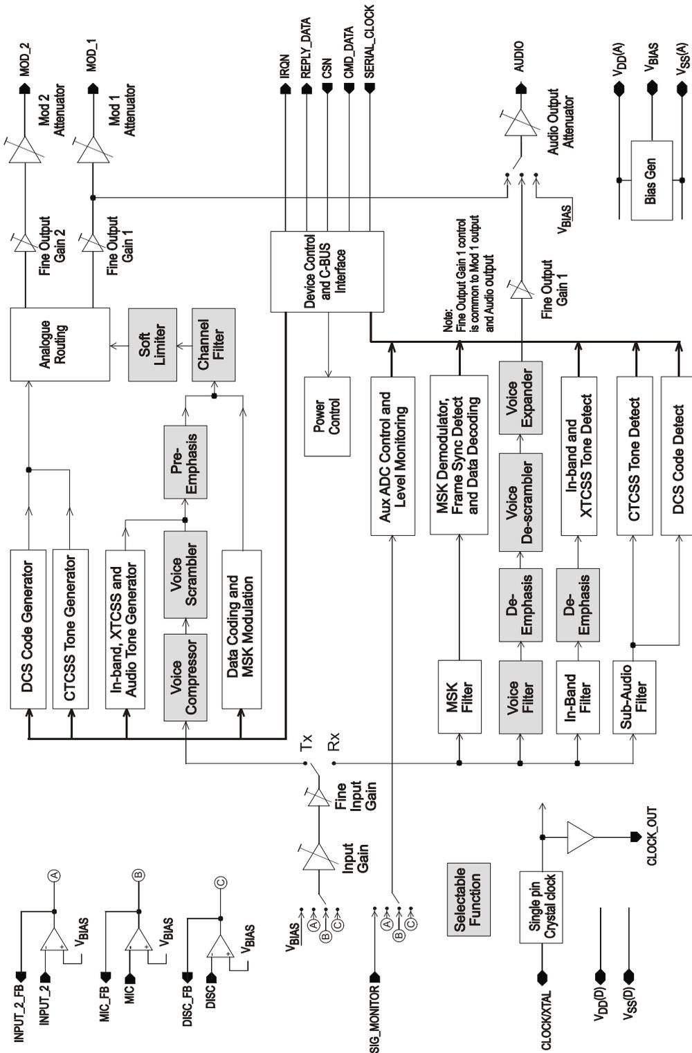
Figure 1 Block Diagram
