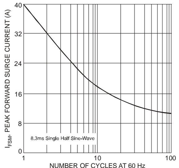
Fig. 6 Maximum Non-Repetitive Peak Forward Surge Current
