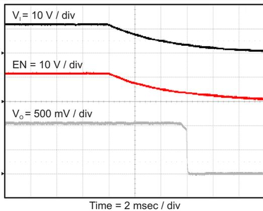
Figure 33. Tps562200 Shut Down Relative To V<sub>1</sub>
