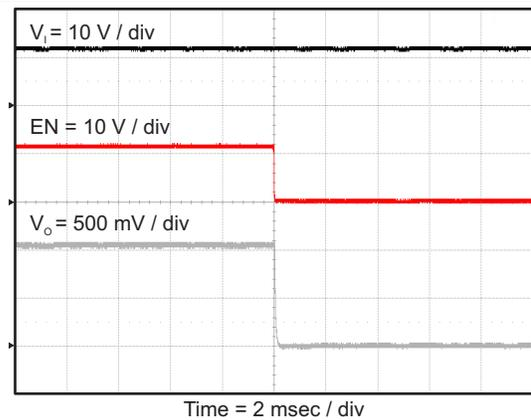
Figure 34. Tps562200 Shut Down Relative To En
