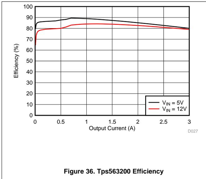
**Figure 36. Tps563200 Efficiency**
