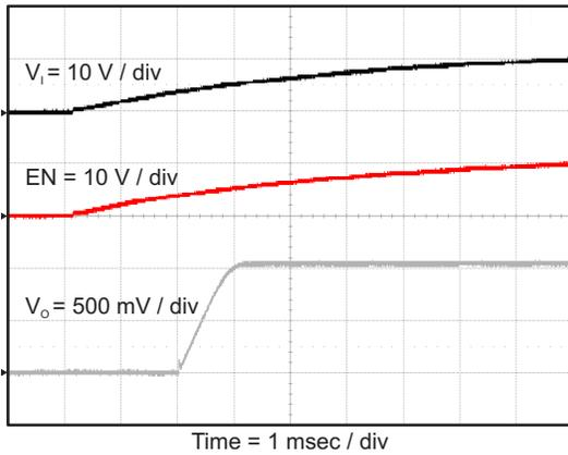
Figure 46. Tps563200 Start Up Relative To  $V_I$
