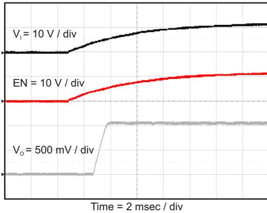
Figure 31. Tps562200 Start Up Relative To V<sub>1</sub>
