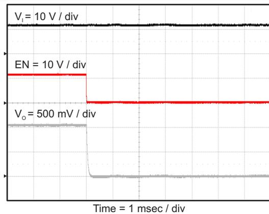
Figure 49. Tps563200 Shut Down Relative To En
