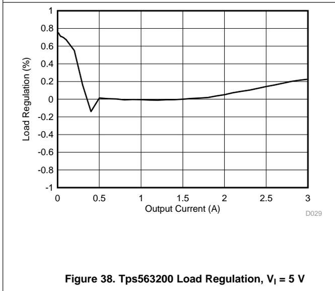
**Figure 38. Tps563200 Load Regulation, V<sub>I</sub> = 5 V**
