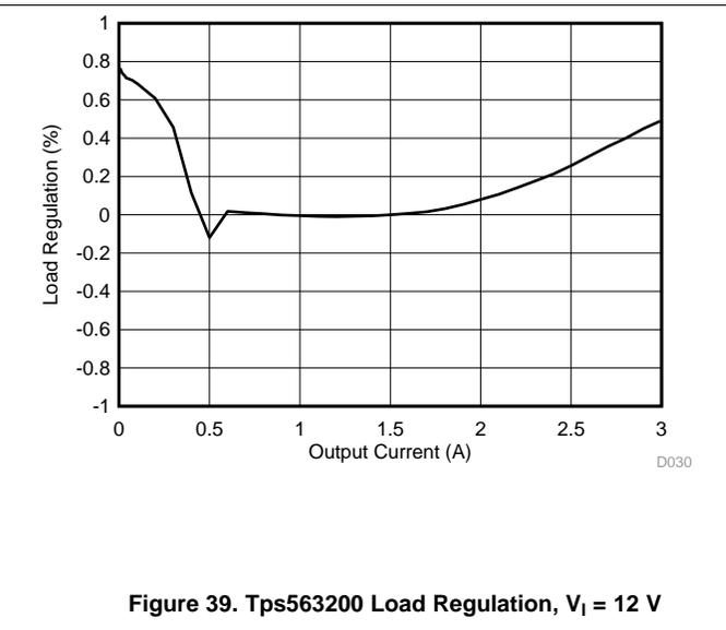
**Figure 39. Tps563200 Load Regulation, V<sub>I</sub> = 12 V**
