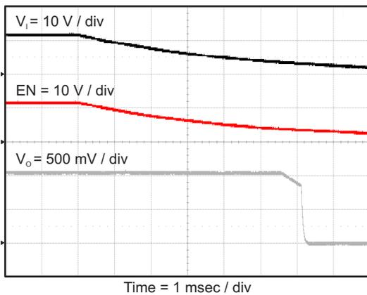
Figure 48. Tps563200 Shut Down Relative To  $V_I$
