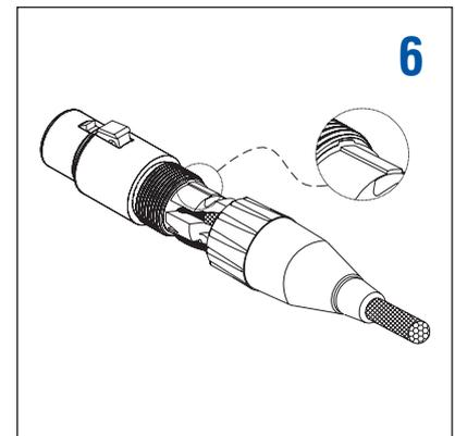
Close the cable clamp slightly and push the boot over the clamp ensuring the wires fit inside the boot.
