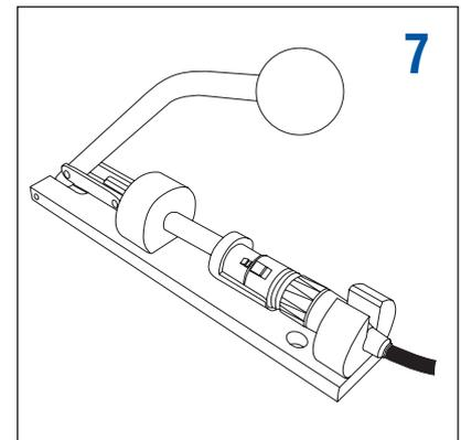
Final assembly can be achieved either by manually screwing the boot on, or by using an Amphenol Australia T2860 termination tool.
