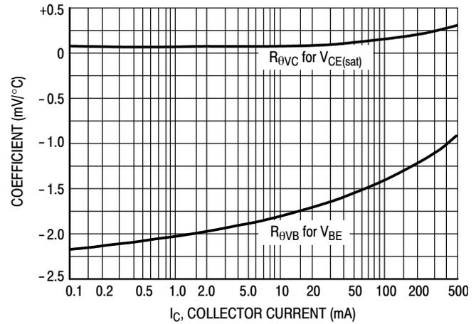
Figure 14. Temperature Coefficients
