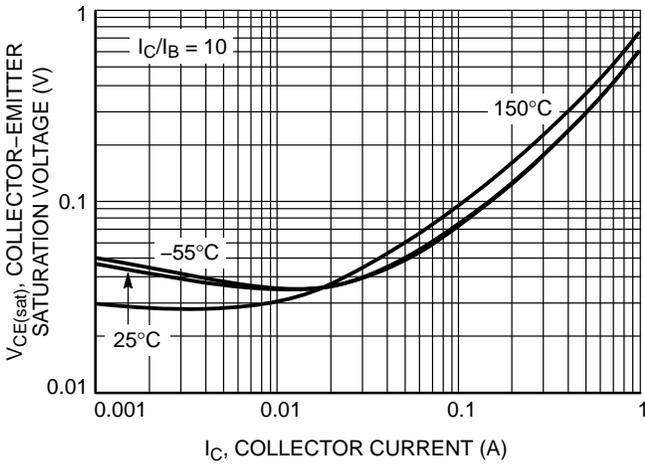
Figure 11. Collector-Emitter Saturation Voltage vs. Collector Current
