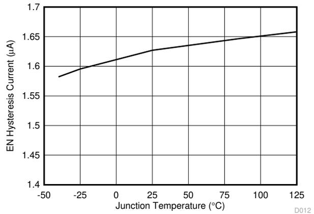
**Figure 6-12. EN Hysteresis Current vs Junction Temperature**
