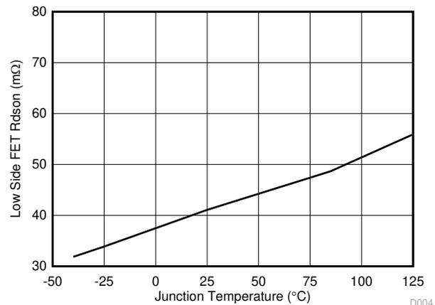
**Figure 6-4. Low-Side FET On Resistance vs Junction Temperature**
