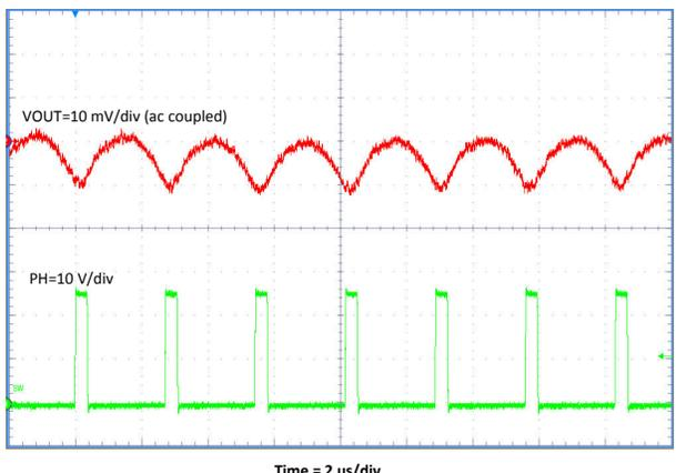
**Figure 8-6. Output Voltage Ripple**
