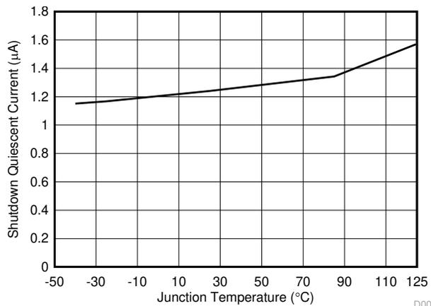
**Figure 6-1. Shutdown Quiescent Current vs Junction Temperature**
