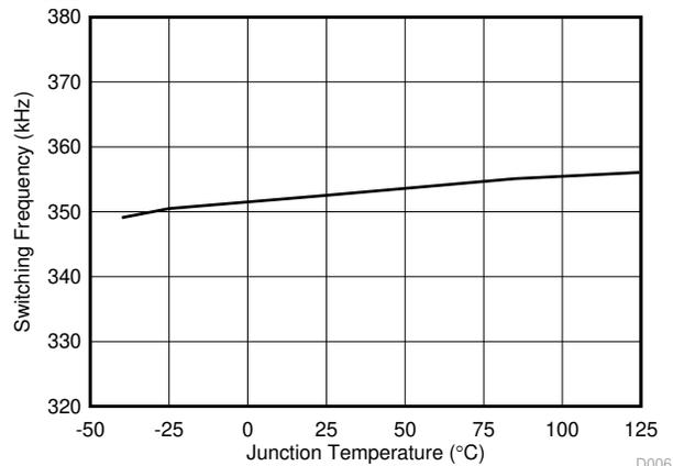
**Figure 6-6. Centre Switching Frequency vs Junction Temperature**
