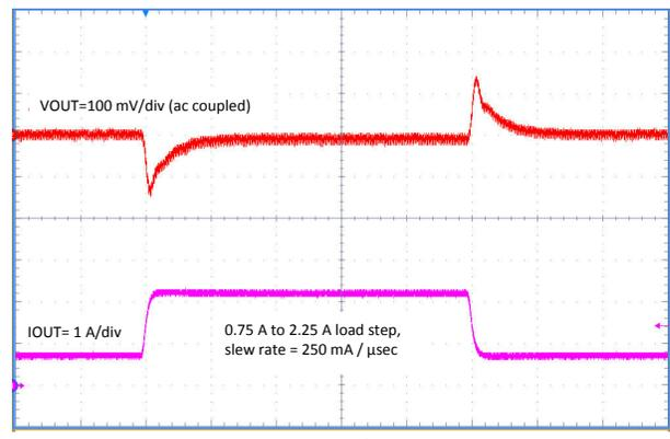
0.75 to 2.25-A load step, slew rate = 250 mA/μsec
