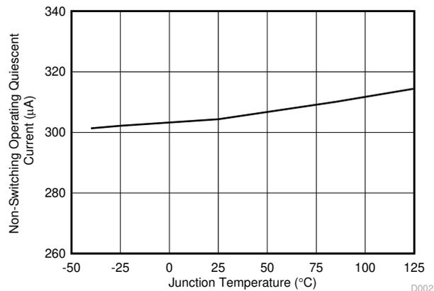
**Figure 6-2. Non-Switching Operating Quiescent Current vs Junction Temperature**
