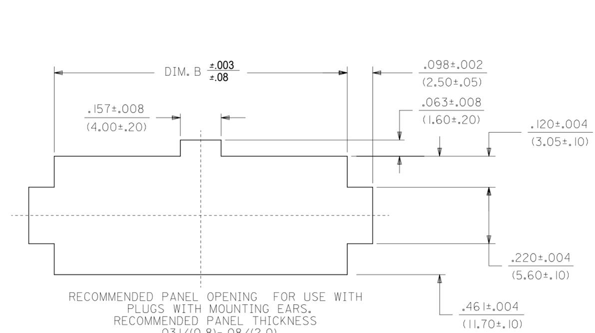
RECOMMENDED PANEL OPENING FOR USE WITH PLUGS WITH MOUNTING EARS.
