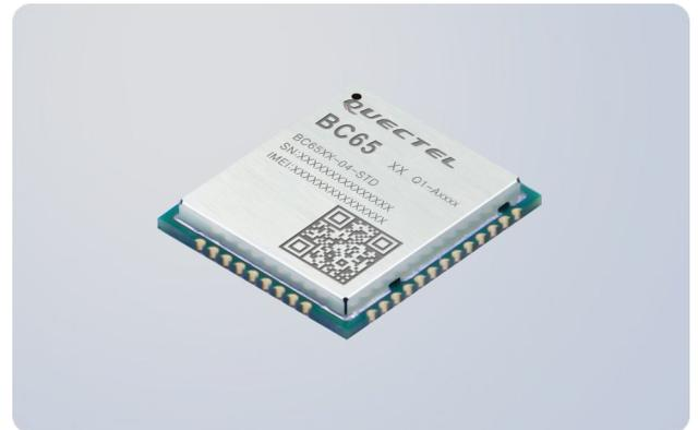
BC65 is high-performance multi-band NB-IoT module with extremely low power consumption. The ultra-compact 17.7mm × 15.8mm × 2.2mm profile makes it a perfect choice for size sensitive applications. Designed to be compatible with Quectel GSM/GPRS M66 , NB-IoT BC66 and BC68 modules in the compact and unified form factor, BC65 provides a flexible and scalable platform for migrating from GSM/GPRS to NB-IoT network.
