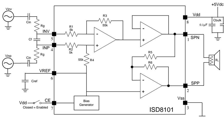
Figure 8-2 ISD8101 Application Diagram
