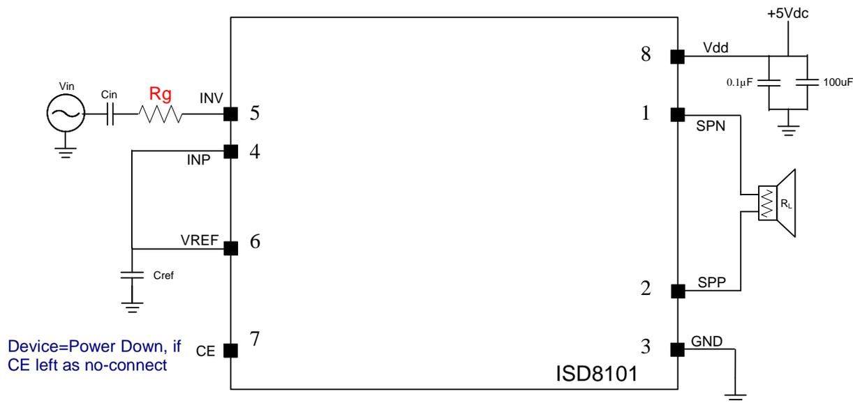
$$\text{Differential Output Gain (SPP - SPN)} = 2x \frac{50k}{5k + R_g}$$
