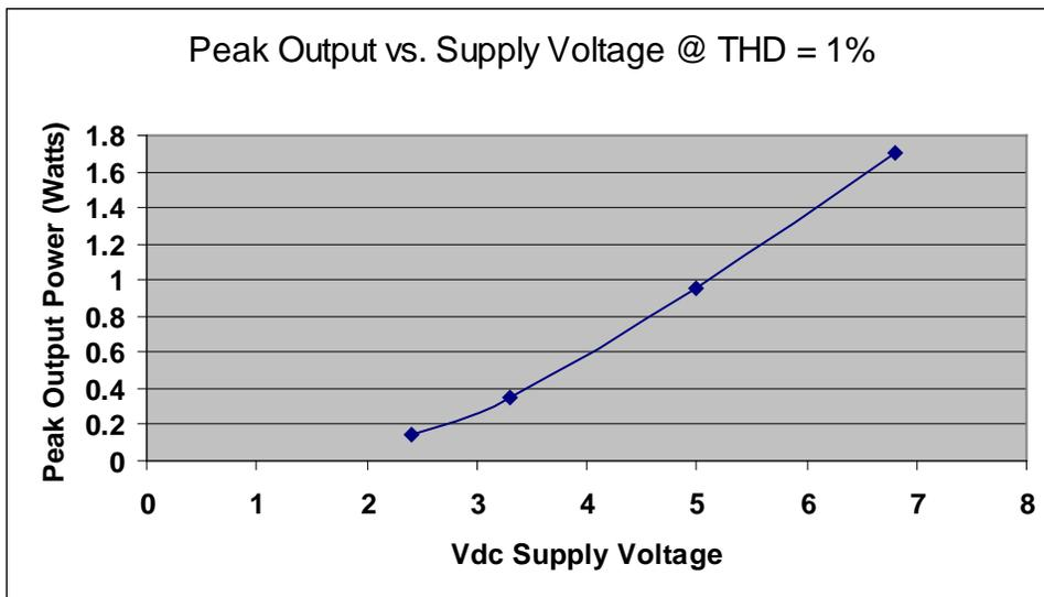
**Note:** Peak output power becomes reduced as device becomes heated. Sustained medium duration heating typical for audio limits maximum useable output to approximately 1.5Wrms at less than 10% distortion.
