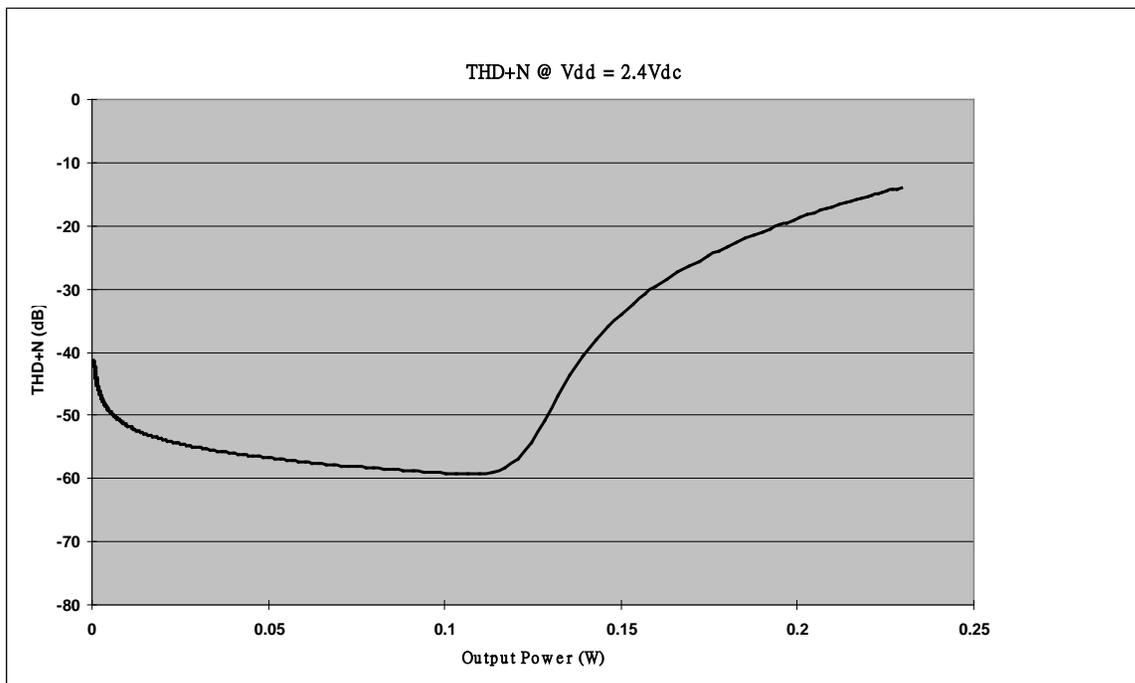
Conditions: THD+N measurement Bandwidth 22Hz to 22kHz at T<sub>A</sub>=25°C
