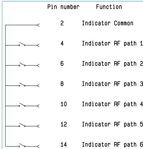
**Ways 1 and 4 are not connected for SP4T switches.**
