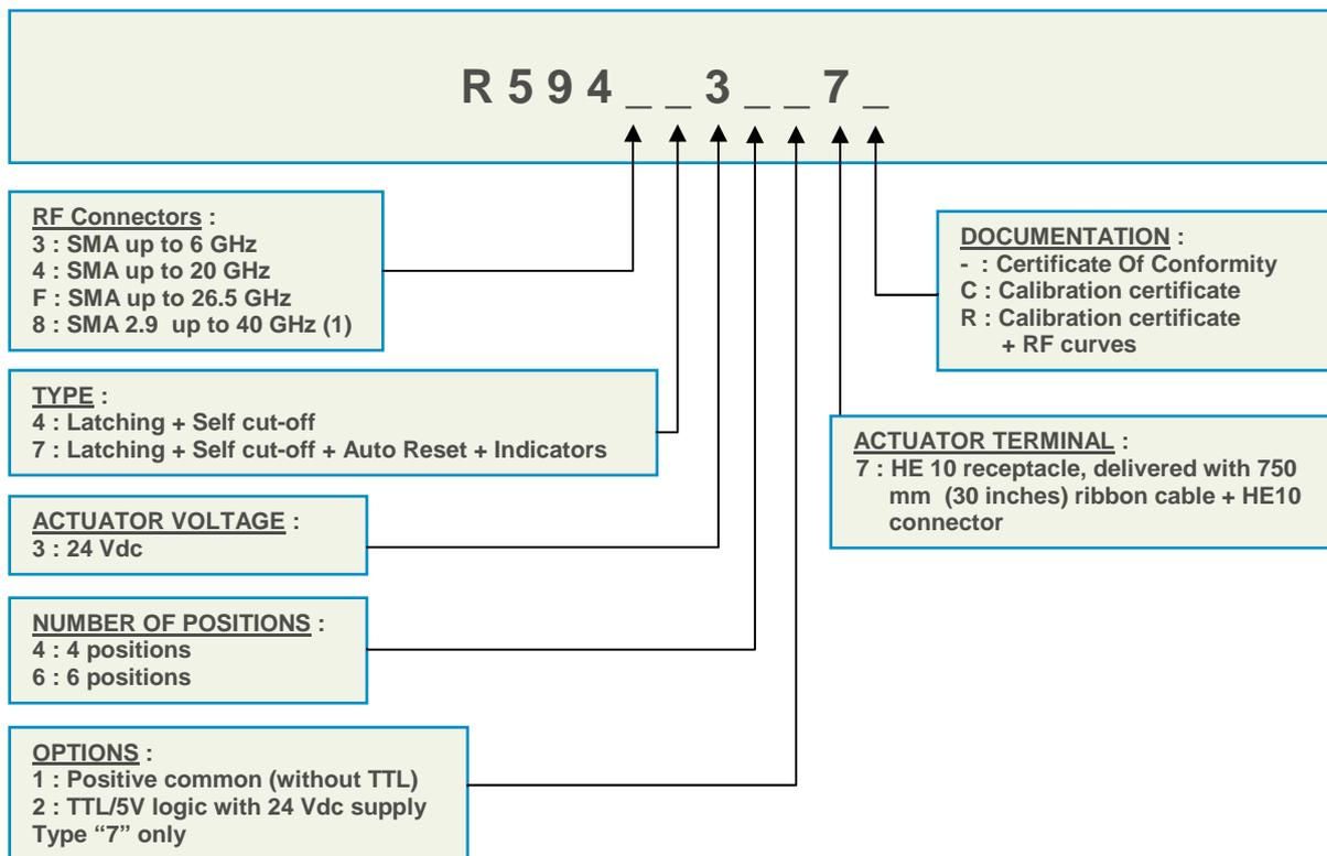
(1) Connector SMA2.9 is equivalent to "K Connector<sup>®</sup>", registered trademark of Anritsu
