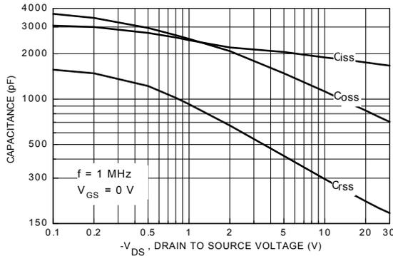
**Figure 9. Capacitance Characteristics.**
