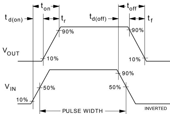
**Figure 12. Switching Waveforms.**
