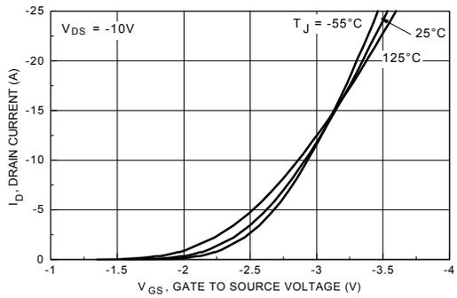
Figure 5. Transfer Characteristics.
