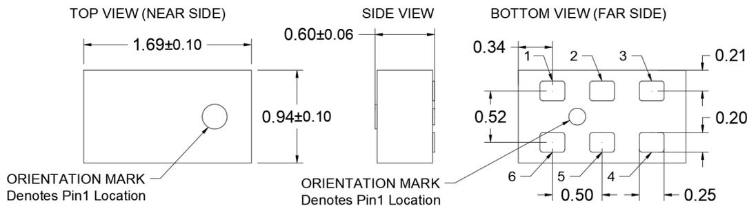
Dimensions are in Millimeters
