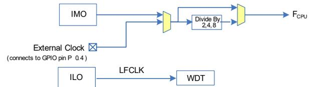
The  $F_{CPU}$  signal can be divided down to generate synchronous clocks for the analog and digital peripherals. There are four clock dividers for the PSoC 4000, each with 16-bit divide capability. The 16-bit capability allows flexible generation of fine-grained frequency values and is fully supported in PSoC Creator.
