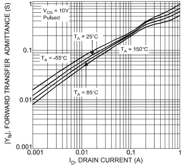
Fig. 10 Forward Transfer Admittance vs. Drain Current
