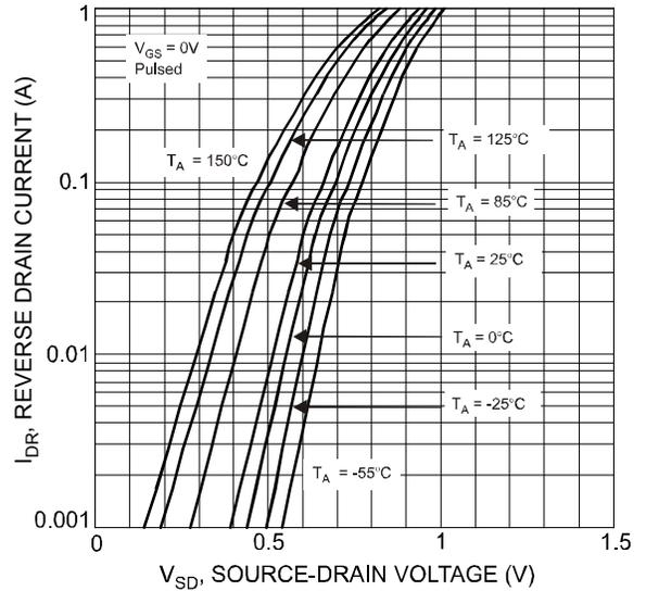
Fig. 8 Reverse Drain Current vs. Source-Drain Voltage
