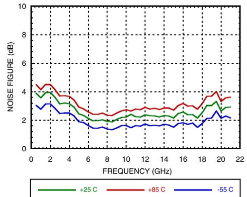
**GaAs PHEMT MMIC LOW NOISE AMPLIFIER, DC - 20 GHz**
