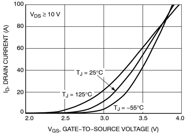
Figure 2. Transfer Characteristics
