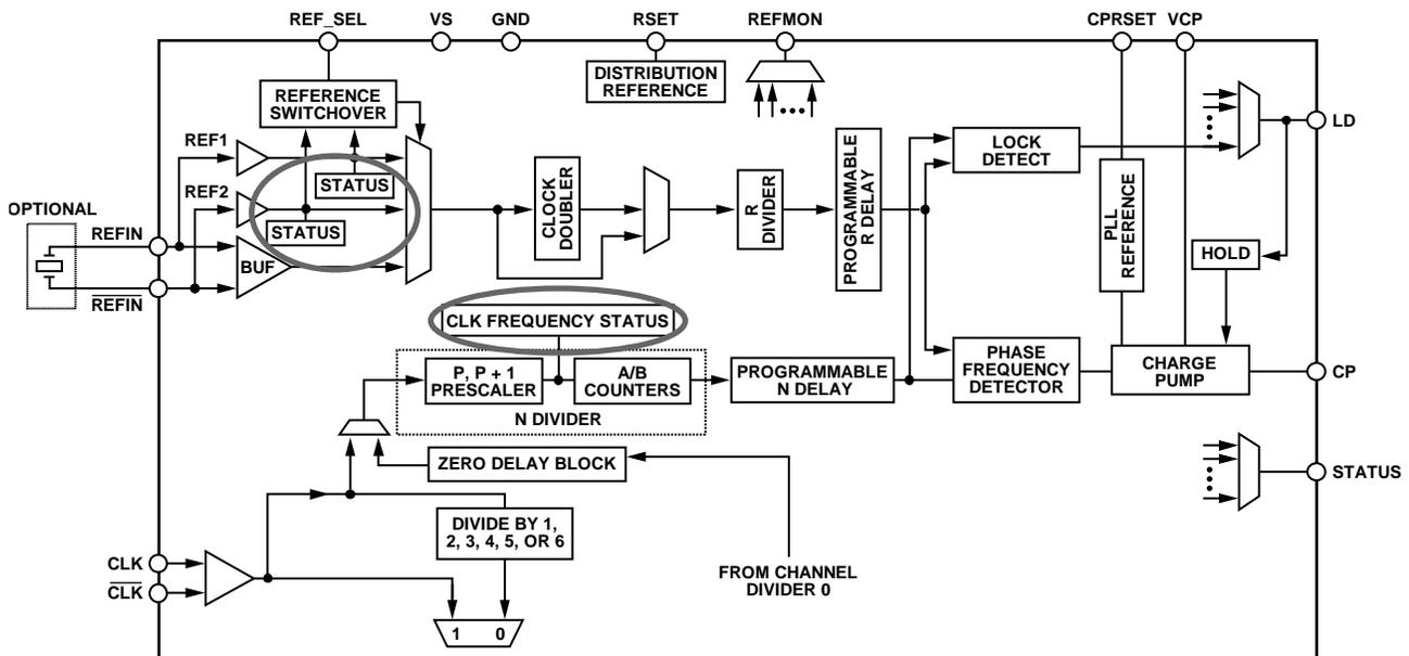
Figure 35. Reference and CLK Frequency Status Monitors
