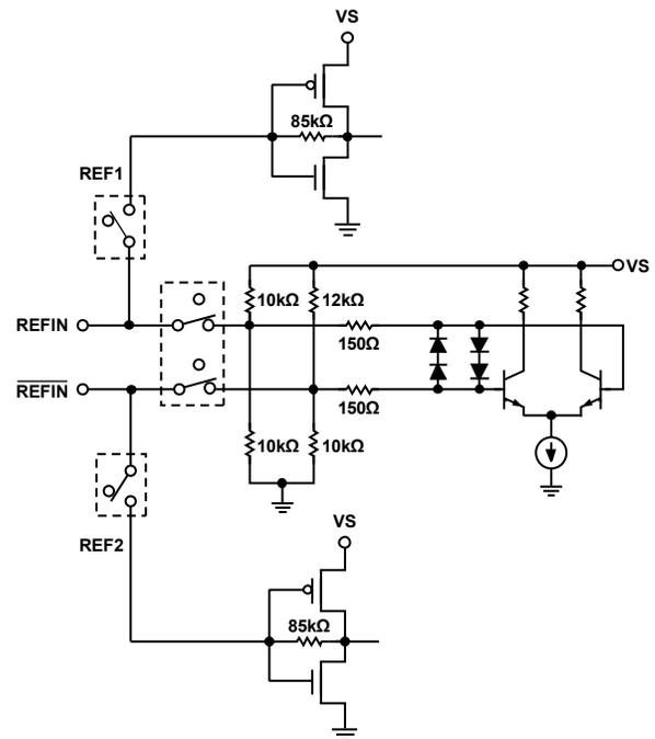
Figure 30. REF1 Equivalent Circuit for Non-XTAL Mode
