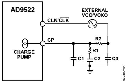
Figure 29. Example of External Loop Filter for PLL
