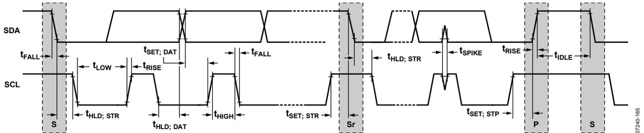
Figure 48. I<sup>2</sup>C Serial Port Timing
