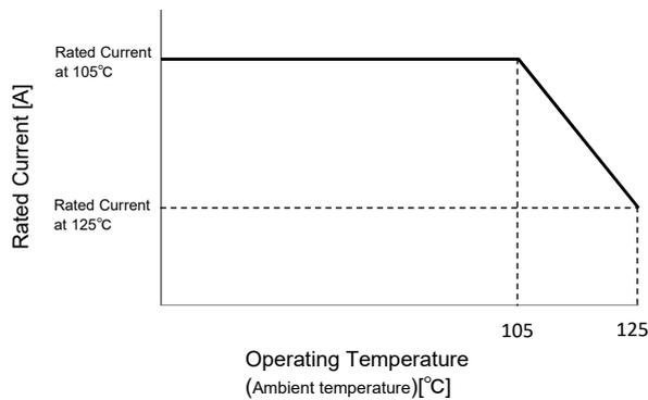
· Operating Temperature : - 40 °C to + 125 °C    · Storage Temperature : - 40 °C to + 125 °C
