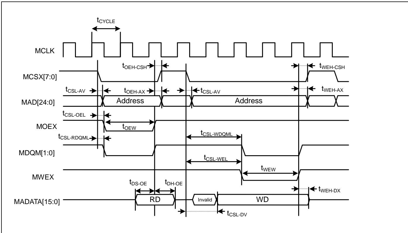
**Separate Bus Access Synchronous SRAM Mode**
