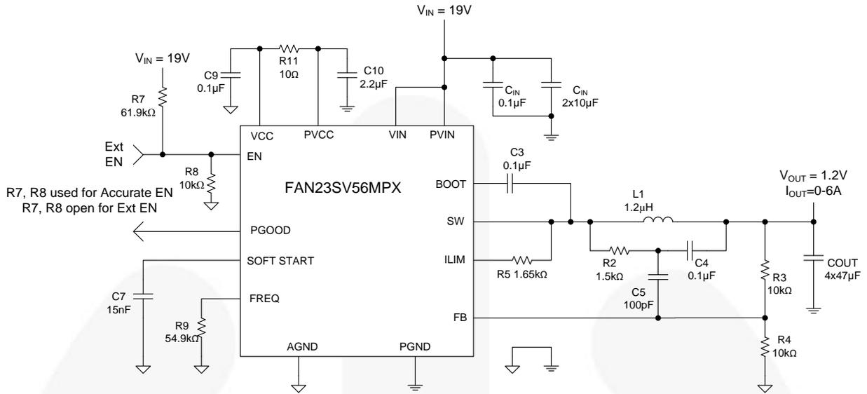
Figure 1. Typical Application with  $V_{IN} = 19V$
