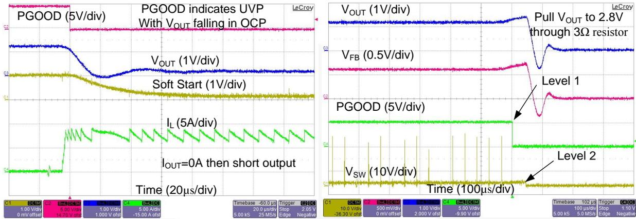
Figure 24. Over-Current Protection with Heavy Load Applied
