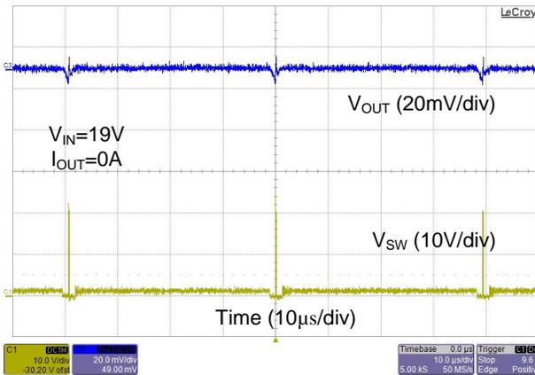
Figure 18. Static Load Ripple at Light Load
