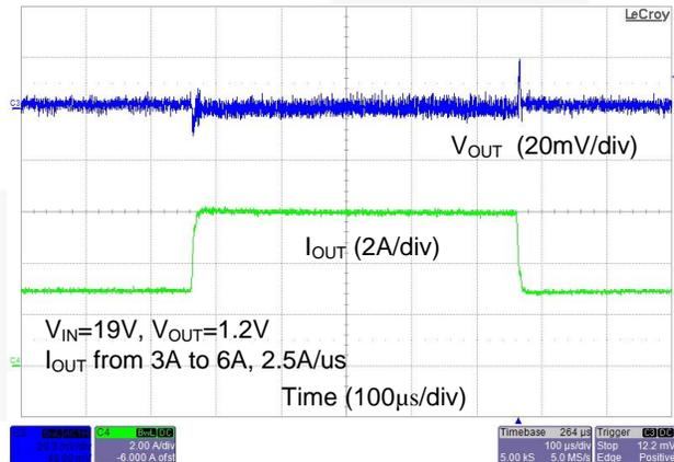
Figure 23. Load Transient from 50% to 100% Load Current
