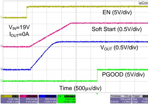
Figure 14. Startup Waveforms with 0 A Load Current
