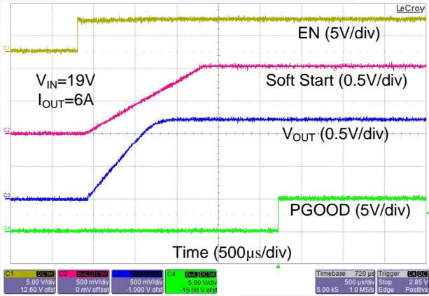
Figure 15. Startup Waveforms with 10 A Load Current
