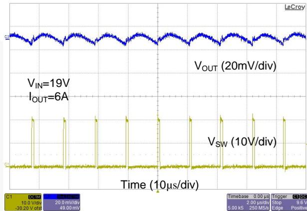
Figure 19. Static Load Ripple at Full Load
