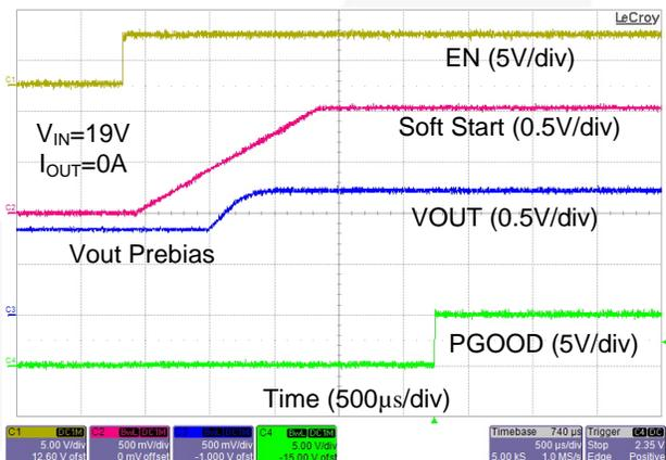
Figure 17. Startup Waveforms with Pre-bias Voltage on Output
