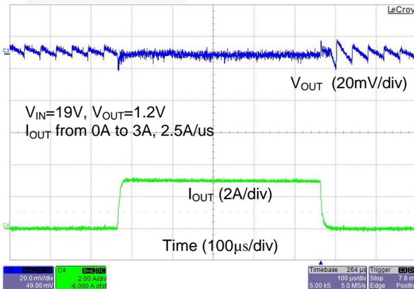
Figure 22. Load Transient from 0% to 50% Load Current
