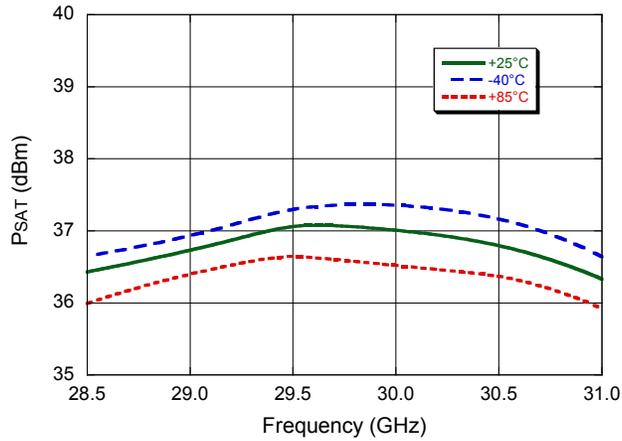
**$P_{SAT}$  vs. Frequency over Bias Voltage**
