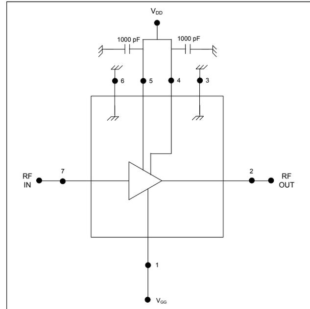
3. Nominal bias is obtained by first connecting  $-5$  volts to pin 1 ( $V_{GG}$ ), followed by connecting  $+8$  volts to pin 5 ( $V_{D1}$ ) and pin 4 ( $V_{D2}$ ). Note sequence.
