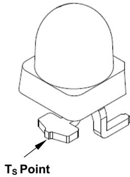
$T_S$  can be easily measured by mounting a thermocouple on the soldering joint as shown in [Figure 15](#), while  $R_{\theta J-S}$  is provided in the data sheet. Verify the  $T_S$  of the LED in the final product to ensure that the LEDs are operating within all maximum ratings stated in the data sheet.
