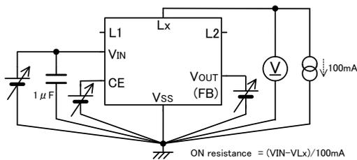
ON resistance =  $(V_{IN} - V_{Lx}) / 100\text{mA}$
