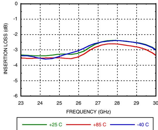
**Insertion Loss RFIN to RF4 vs. Temperature**
