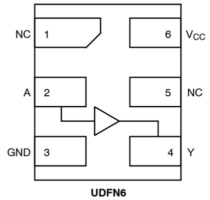
Figure 2. Pinout (Top View)
