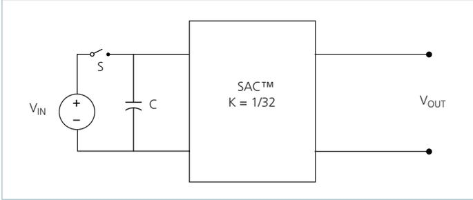
Figure 19 — Sine Amplitude Converter™ with input capacitor
