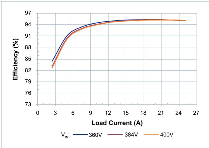
Figure 9 — Efficiency at  $T_{CASE} = 100^{\circ}C$
