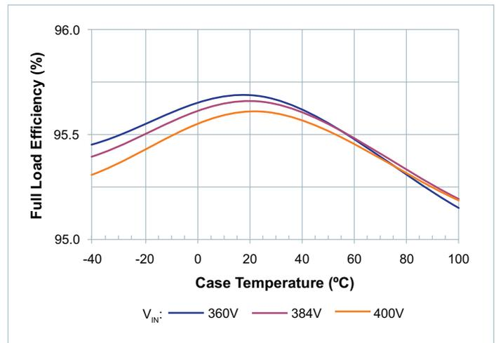
Figure 4 — Full load efficiency vs. temperature;  $V_{IN}$
