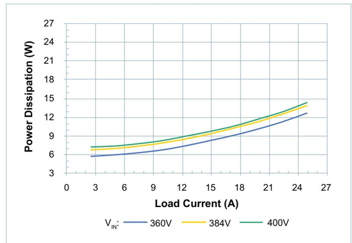
Figure 8 — Power dissipation at  $T_{CASE} = 25^{\circ}C$
