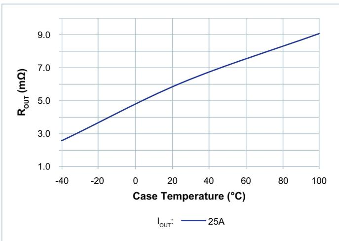
Figure 11 —  $R_{OUT}$  vs. temperature; nominal input
