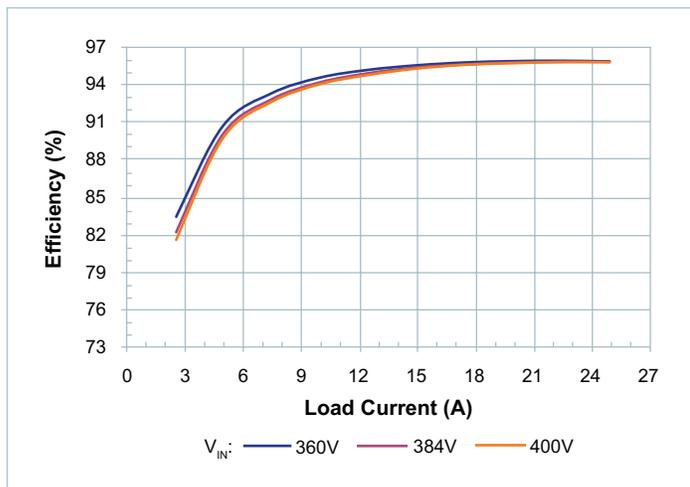
Figure 7 — Efficiency at  $T_{CASE} = 25^{\circ}C$
