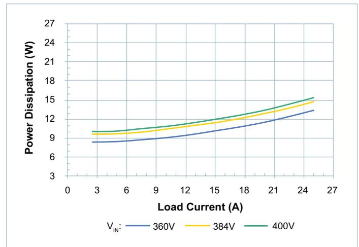
Figure 6 — Power dissipation at  $T_{CASE} = -40^{\circ}C$
