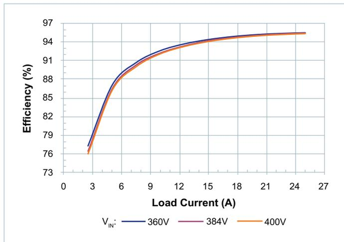
Figure 5 — Efficiency at  $T_{CASE} = -40^{\circ}C$
